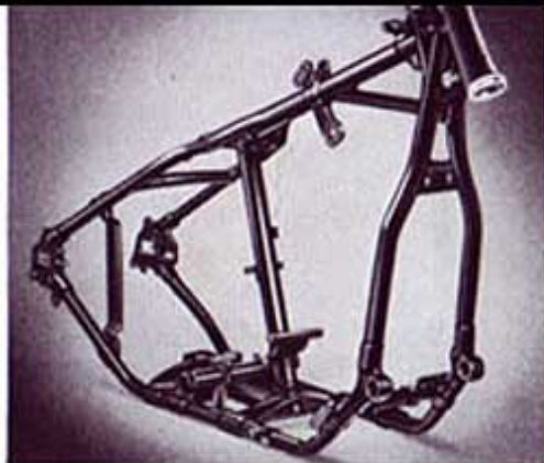
Terminal box lugs and safety guard mounting plate incorporated on new Big Twin frames.
