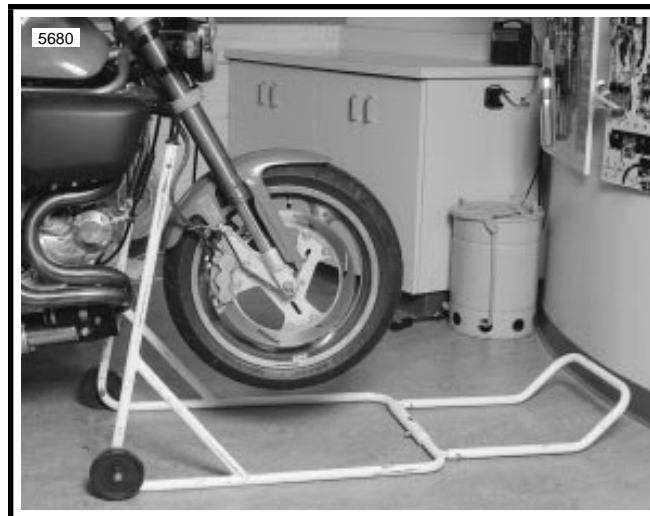
Figure 2-4. Front Wheel Support Stand (Part No. B-41395) with S1 Lift Adapter (Part No. B-41686)
