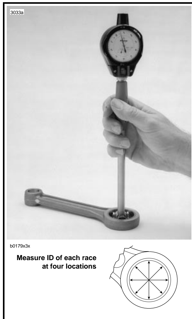
Figure 3-73. Measuring Connecting Rod Race Inside Diameter
