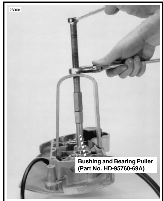
Figure 3-55. Removing Bushing
