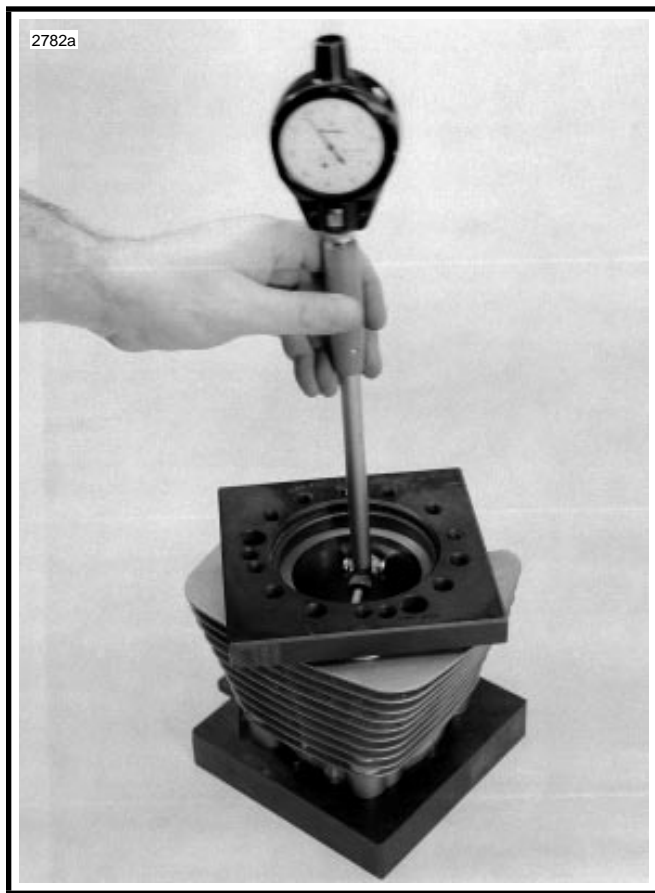
Figure 3-30. Measuring Cylinder Bore Using Torque Plates (Part No. HD-33446A)
