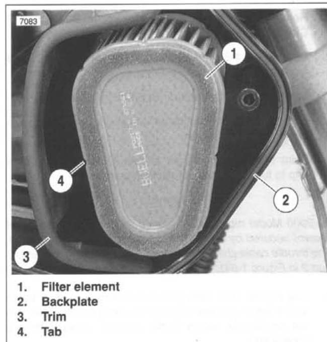
Figure 1-63. Installed Air Cleaner Filter
