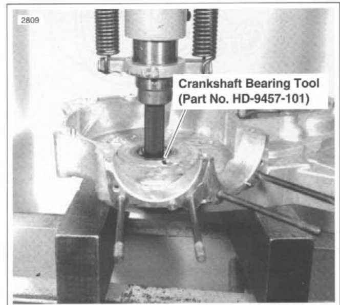
Figure 3-98. Sprocket Shaft Outer Race Removal
