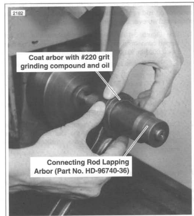
Figure 3-101. Lapping Connecting Rod Races
