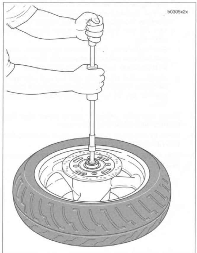
Figure 2-15. Removing Wheel Bearing
