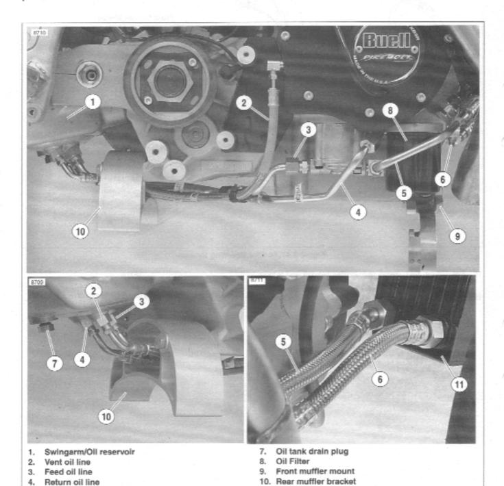
Figure 3-48. Oil Lines and Connections
