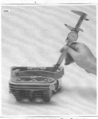
Figure 3-73, Measuring Valve Stem Protrusion
