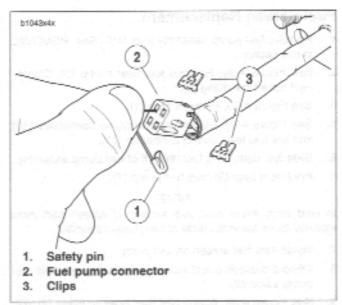
Figure 4-92. Fuel Pump Connector Disassembly
