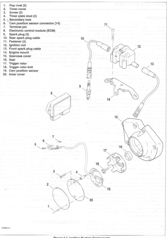
Figure 7-1. Ignition System Components
