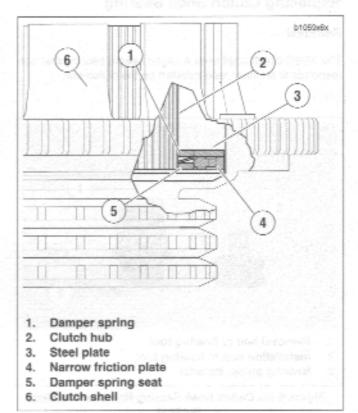
Figure 6-32, Clutch Pack Stack-Up (Cut-Away Vlew)
