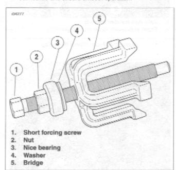
Figure 2-7. Assemble Puller
