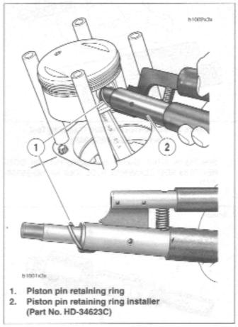
Figure 3-108. Installing Piston Pln Circlip
