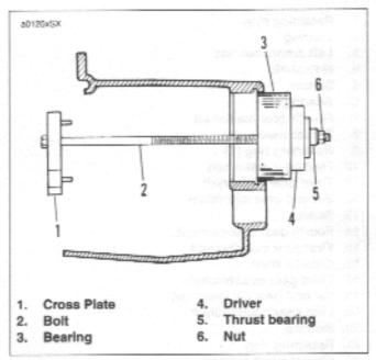
Figure 6-71. Installing Malnshaft Ball Bearing
