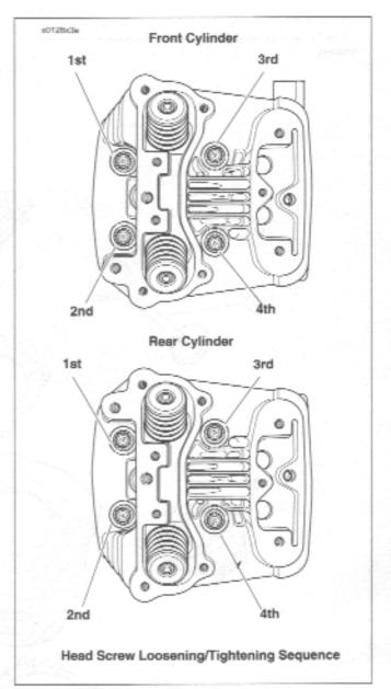
Figure 3-65. Head Screw Loosening/Tightening Sequence
