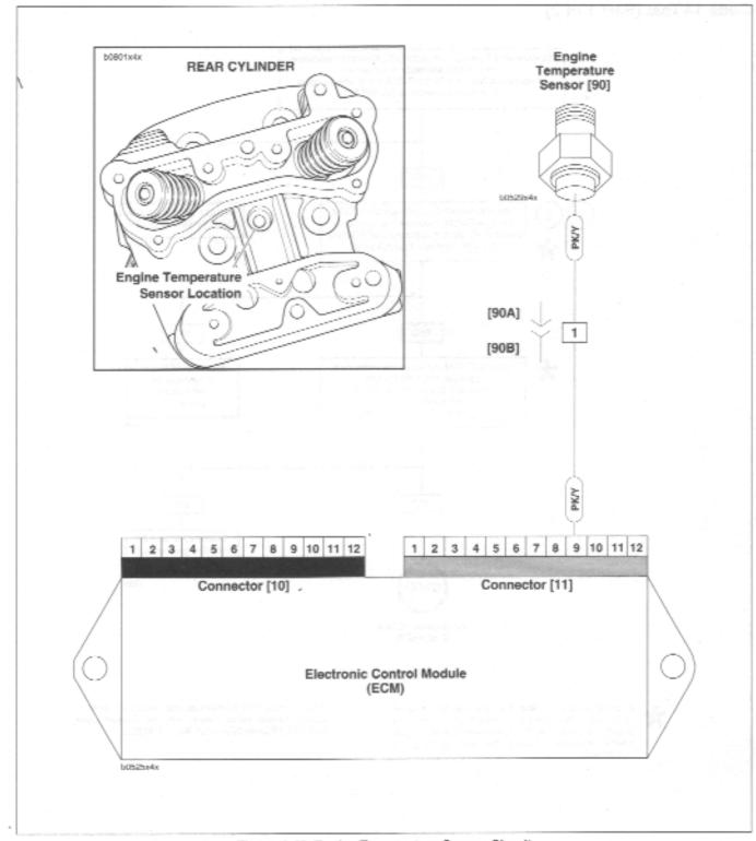
Figure 4-40. Engine Temperature Sensor Circuit
