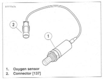
Figure 4-37. Oxygen Sensor
