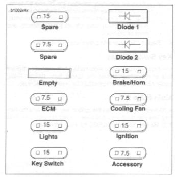
Figure 7-19. Fuses and Diodes
