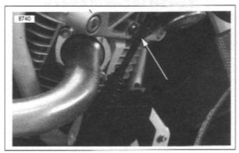
Figure 2-79. Clutch Cable P-clamp
