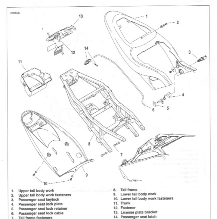
Figure 2-112. Tail Frame and Body Work Assembly
