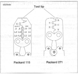
Figure B-15. Packard Terminal Crimp Tools
