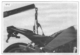
Figure 3-25. Supporting Vehicle for Disassembly
