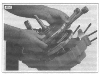
Figure 6-49. Removing Flywheels from Left Case Half
