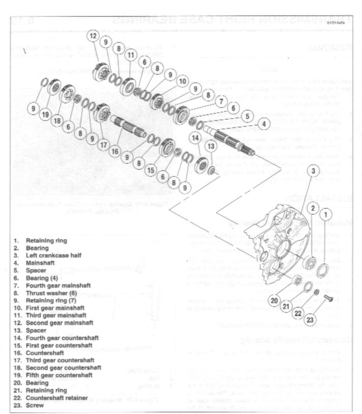
Figure 6-72. Transmission Assembly Left Crankcase Half
