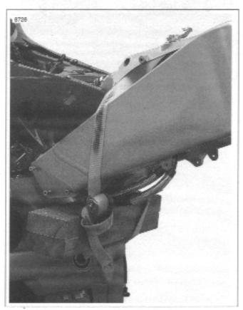
Figure 3-33. Securing Vehicle for Relocation
