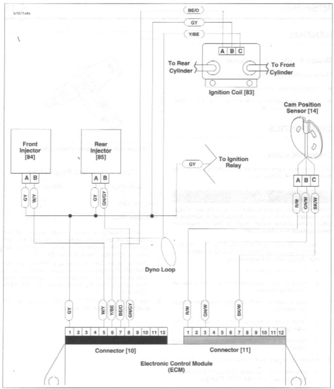
Figure 4-33. Ignition Coil Circuit
