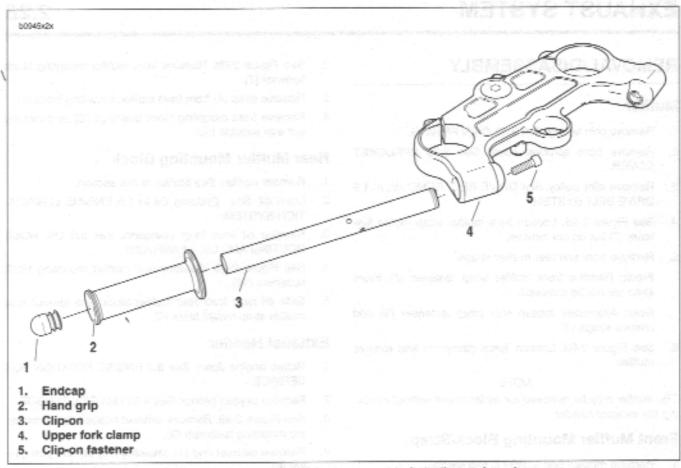
Figure 2-97. Handlebar Clip-on Assembly (left clip-on shown)
