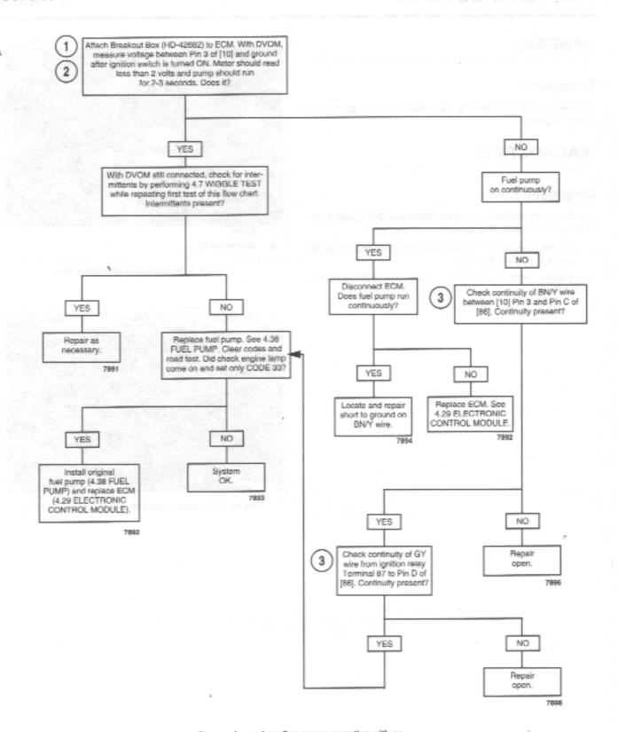
Clear codes and confirm proper operation with no check engine lamp. Codes can be cleared using DIGITAL TECHNICIAN (Part No. HD-44750).
