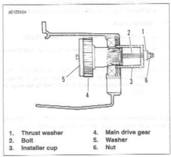
Figure 6-67. Main Drive Gear Installation
