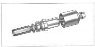
Part No. HD-95970-32D Piston Pin Bushing Tool
