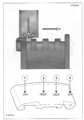
Figure 6-5. Measuring Chain Adjuster Shoe
