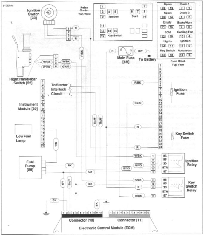
Figure 4-53. Fuel Pump Circuit
