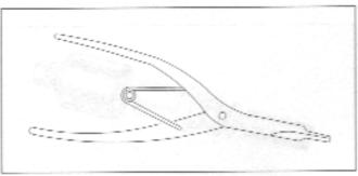
Part No. J-5586 Transmission Shaft Retaining Ring Pliers
