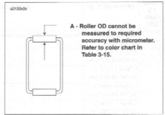
Figure 3-144. Bearing Identification
