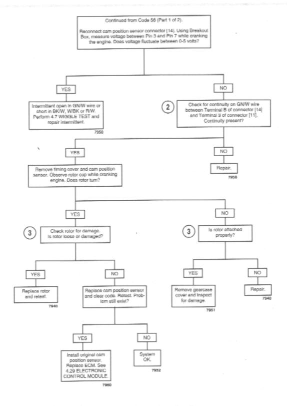
Clear codes and confirm proper operation with no check engine lamp. Codes can be cleared using DIGITAL TECHNICIAN (Part No. HD-44750).
