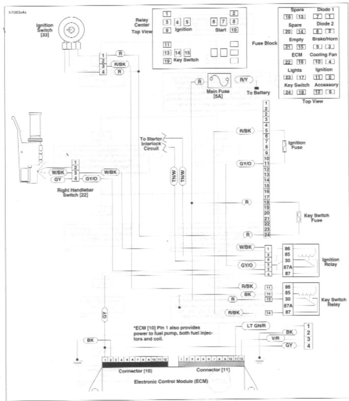
Figure 4-45. Battery Voltage Circuit
