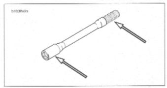
Figure 2-22. Anti-Selze Lubricant Location
