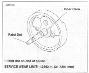
Figure 3-142. Factory Inner Race Sizes
