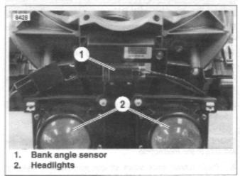
Figure 4-78. Bank Angle Sensor
