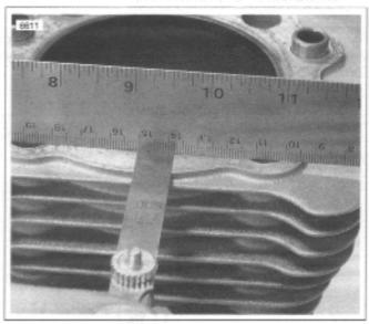
Figure 3-95. Checking Gasket Surfaces
