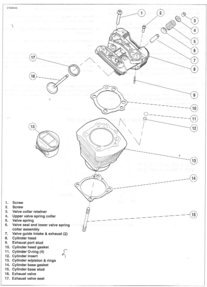
Figure 3-80. Cylinder Head, Cylinder and Piston Assembly
