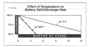
Figure 1-2. Battery Self-Discharge Rate
