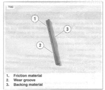
Figure 1-11. Brake Pad Thickness
