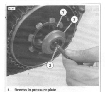
Figure 6-18. Aligning Tabs
