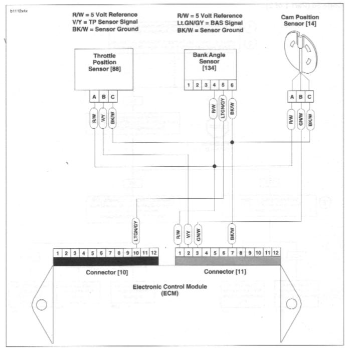
Figure 4-63. Cam Position Sensor Circuit
