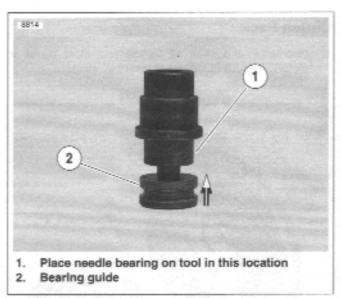
Figure 6-28. Bearing Installer
