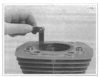
Figure 3-98. Measuring Ring End Gap
