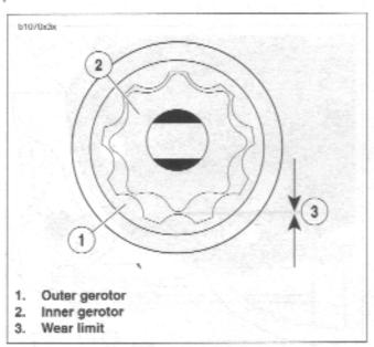
Figure 3-120. Gerotor Wear Limits
