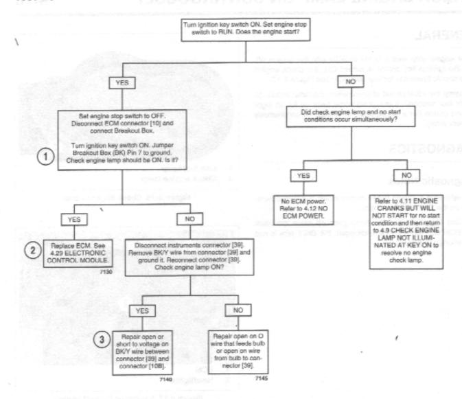
If the engine stop switch is set to RUN with the engine off, and the ignition key switch is turned ON, the check engine lamp should Illuminate for four seconds. See Figure 4-16.
