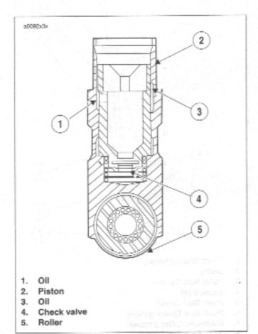
Figure 3-123. Lifter Assembly (Typical)
