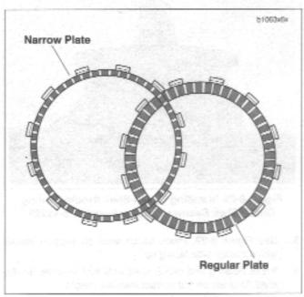
Figure 6-31. Friction Plates
