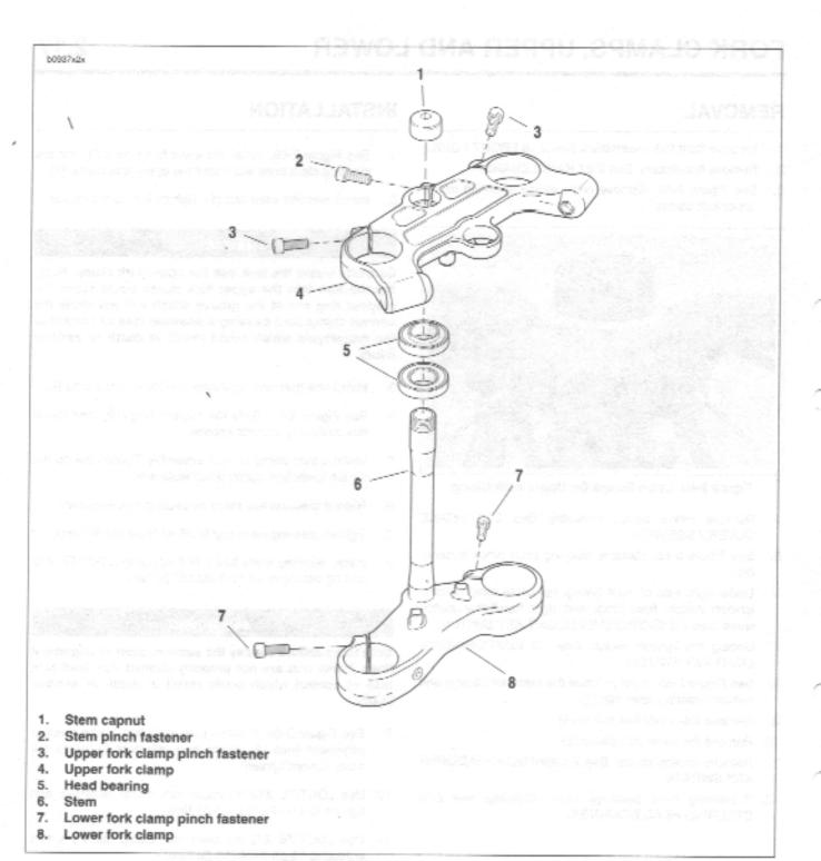
Figure 2-69. Steering Stem Assembly
