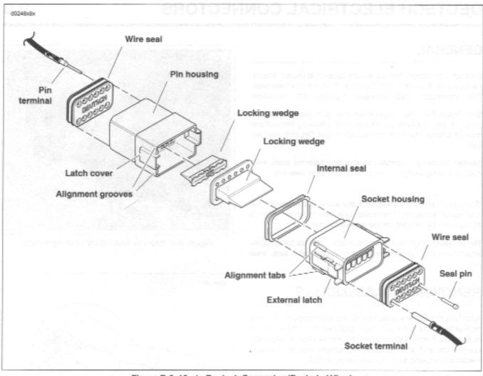
Figure B-8. 12-pin Deutsch Connector (Exploded View)
