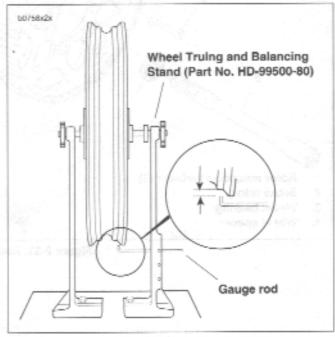
Figure 2-25. Checking Cast Rim Radial Runout
