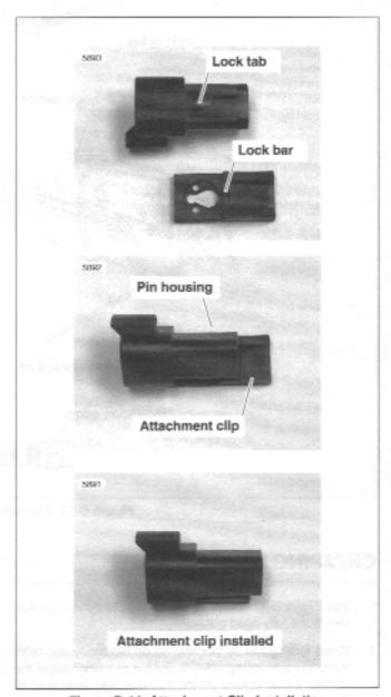
Figure B-11. Attachment Clip Installation
