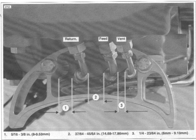
Figure 3-49. Oil Line Clearances and Torques
