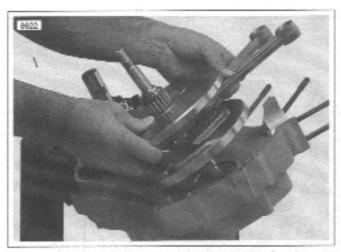
Figure 3-136. Removing Flywheels from Left Crankcase
