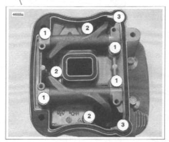
Figure 3-90. Lower Rocker Box Fasteners
