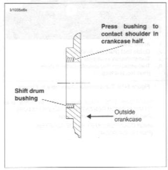
Figure 6-74. Shift Drum Bushing Assembly
