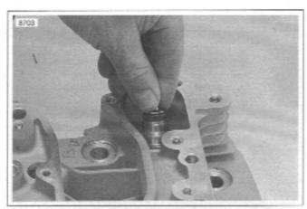
Figure 3-83. Valve Seal and Lower Collar Assembly Installation
