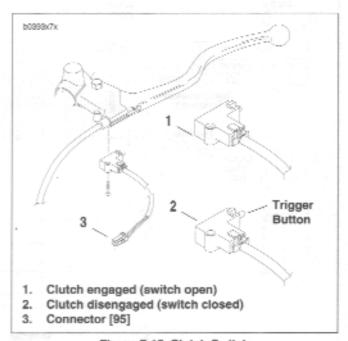
Figure 7-15. Clutch Switch
