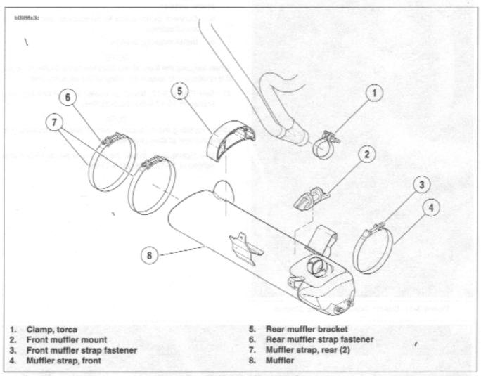
Figure 3-13. Muffler and Mounting System
