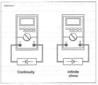
Figure 7-11. Ohmmeter Diode Test
