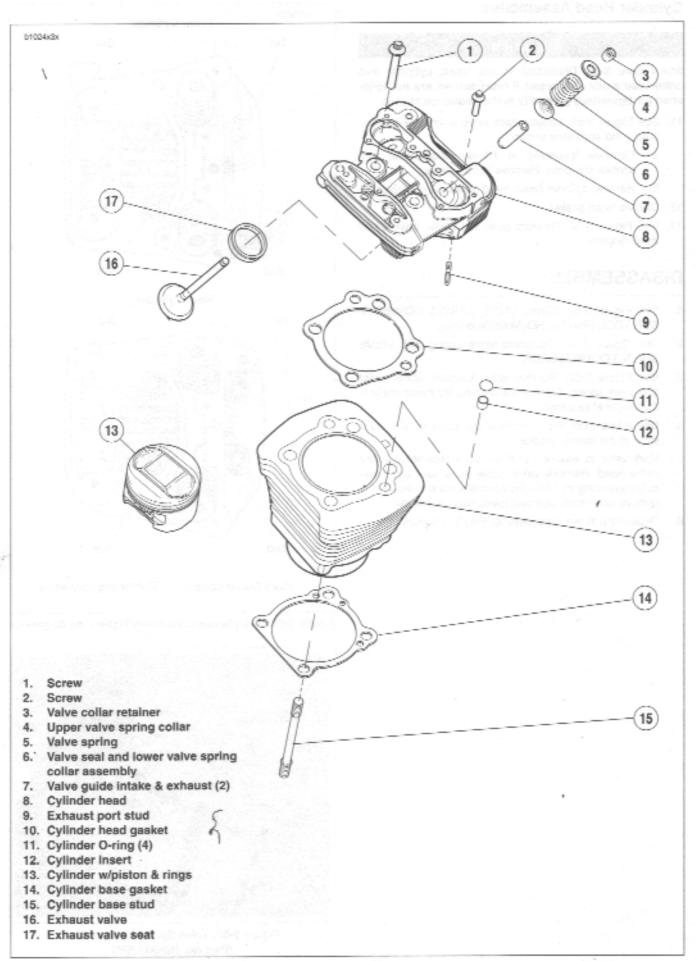
Figure 3-67. Cylinder Head, Cylinder and Piston Assembly
