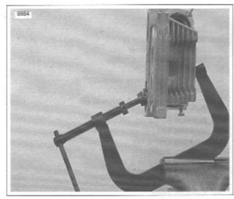
Figure 3-66. Valve Spring Compressor (Part No. HD-34736B)
