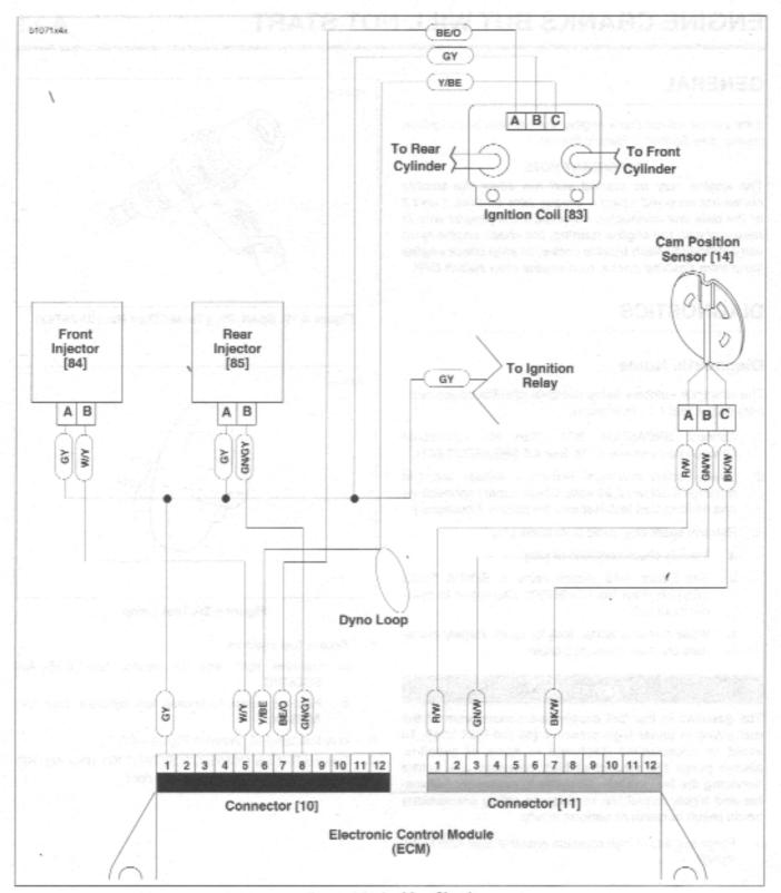
Figure 4-21. Ignition Circuit
