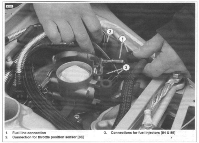
Figure 3-61. Fuel Line and DDFI Electrical Connections
