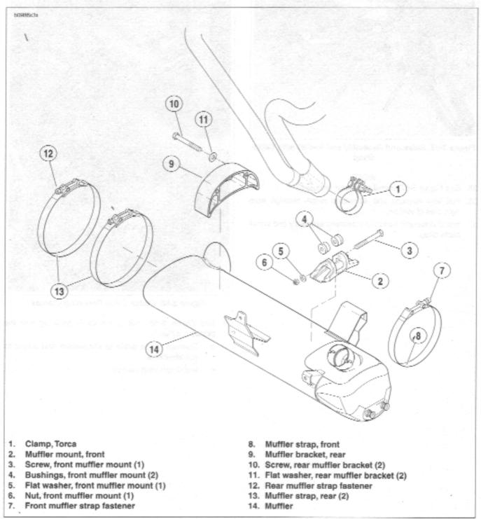
Figure 3-59. Muffler and Mounting System
