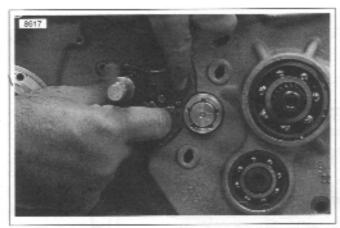
Figure 6-42. Removing Shifter Shaft Assembly
