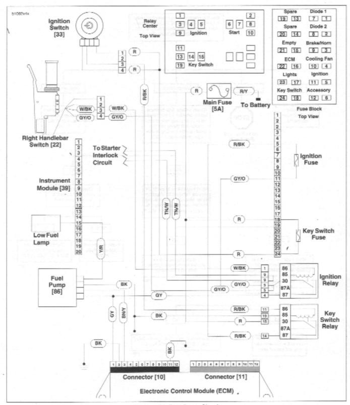
Figure 4-30. Fuel Pump Circuit
