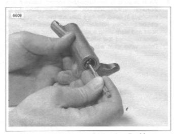
Figure 3-72. Measuring Rocker Arm Bushing Inner Diameter
