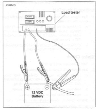
Figure 7-24. Check Current Draw (Ignition Switch On)
