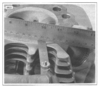
Figure 3-68. Checking Gasket Surface
