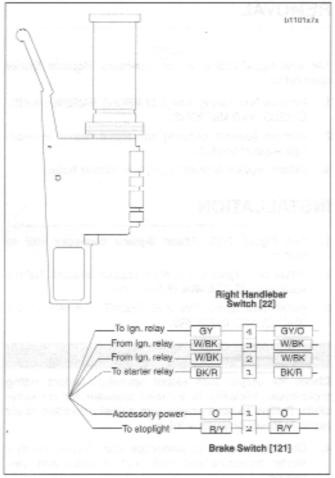
Figure 7-52. Right Handlebar Switch Connection
