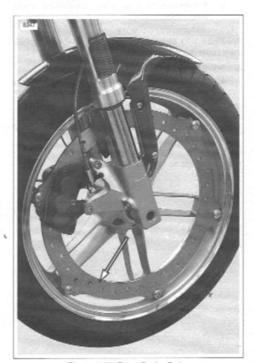
Figure 1-12. Front Brake Rotor
