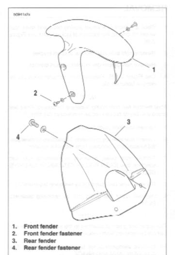
Figure 2-104. Front and Rear Fender
