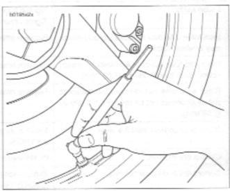
Figure 2-4. Checking Tire Inflation Pressure
