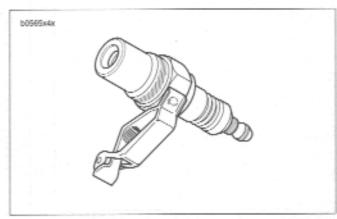
Figure 4-19. Spark Plug Tester (Part No. HD-26792)
