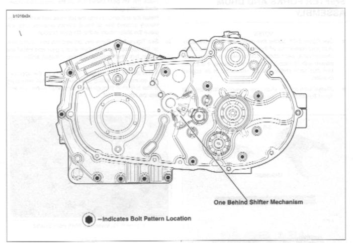
Figure 6-79. Crankcase Fasteners
