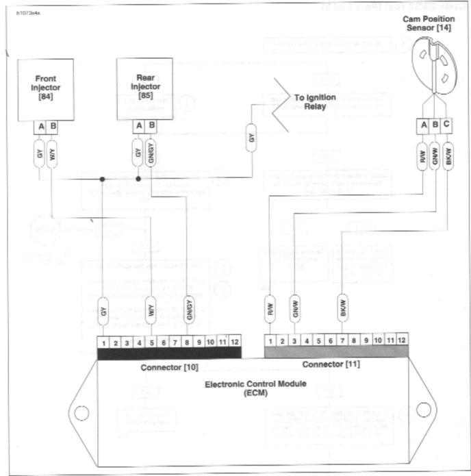
Figure 4-48. Fuel Injector Circuit
