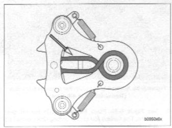
Figure 6-84. Shifter Shaft Return Spring (Correctly Installed)
