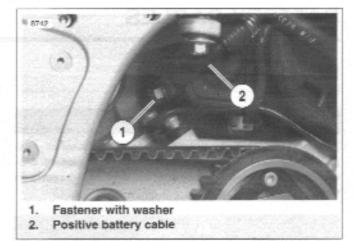
Figure 7-37. Positive Battery Cable (Protective Boot Not Shown)
