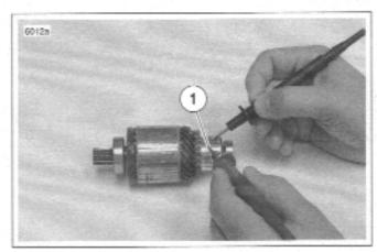
Figure 5-20. Open Armature Test
