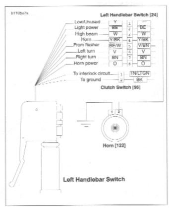
Figure 7-65. Horn Wiring
