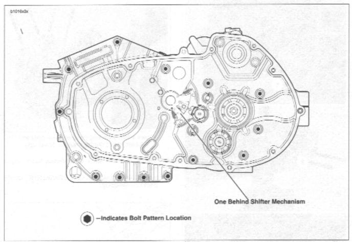
Figure 3-153. Crankcase Fasteners
