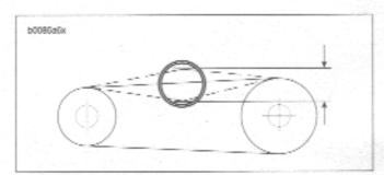
Figure 1-29. Measuring Primary Chain Tension
