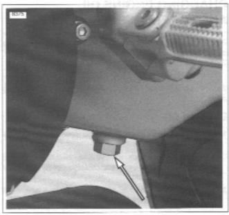
Figure 1-3. Oil Tank Drain Plug
