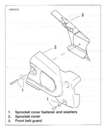
Figure 2-103. Sprocket Cover
