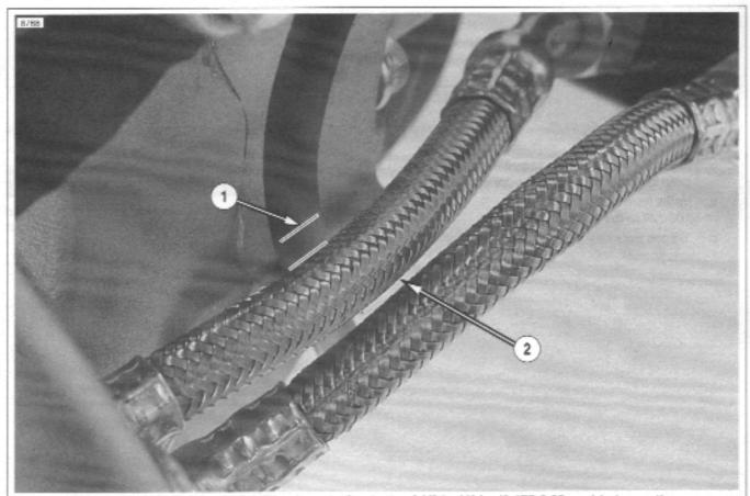
Verify that the clutch cable and feed line have a clearance of 1/8 to 1/4 in. (3.175-6.35 mm) between them.
