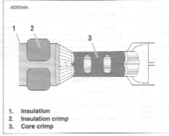
Figure B-16. Inspect Core and Insulation/Seal Crimps
