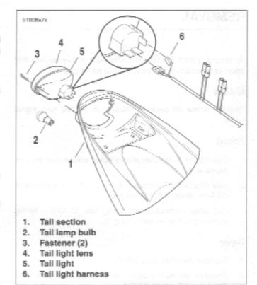
Figure 7-45. Tail Lamp Assembly
