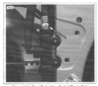
Figure 2-50. Rear Brake Line Switch/Banjo Bolt
