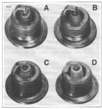
Figure 1-44. Typical Spark Plug Deposits
