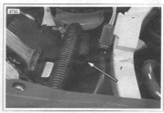
Figure 3-28. Transmission Vent Line
