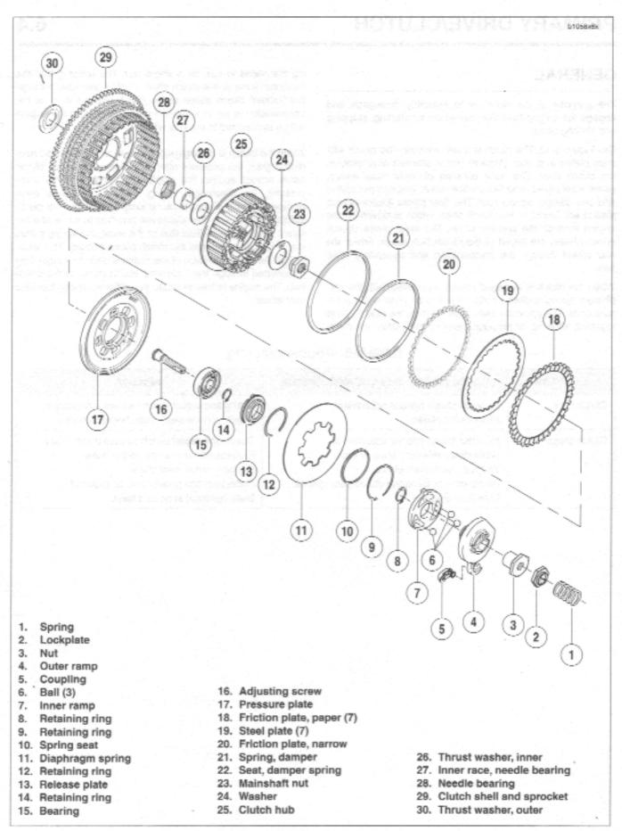
Figure 6-12. Clutch Assembly
