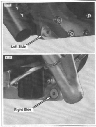
Figure 3-31. Front Exhaust Mount Bushings (2 piece)
