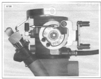
Figure 4-115. Emissions Hose Attachment, California Models Only
