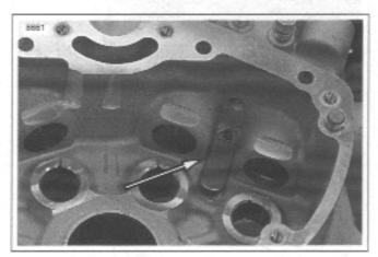
Figure 3-114. Reed Valve Assembly in Gearcase
