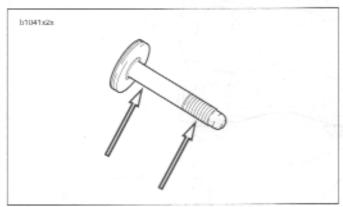
Figure 3-45. Lubrication Points on Front Isolator Bolt
