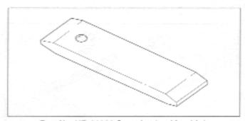
Part No. HD-38362 Sprocket Locking Link
