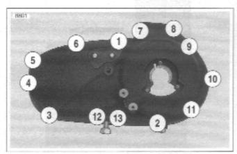
Figure 6-6. Primary Cover Tightening Sequence
