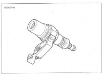
Figure 4-32. Spark Tester (Part No, HD-26792)
