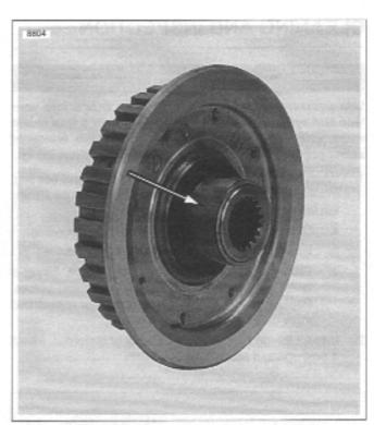
Figure 6-25. Clutch Hub Bearing Race
