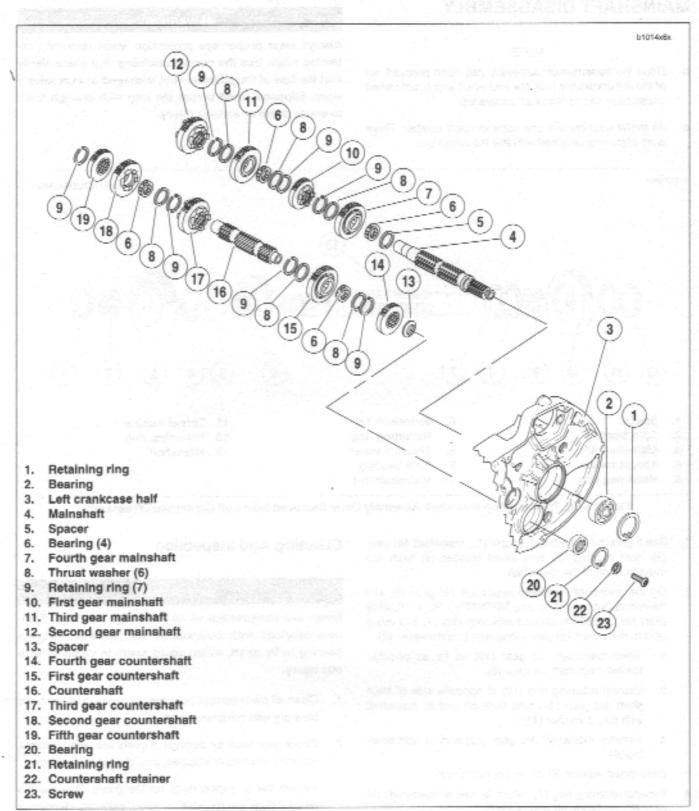
Figure 6-57. Transmission Assembly-Left Crankcase Half
