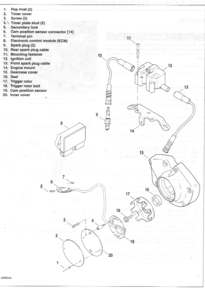
Figure 4-68. Ignition Components
