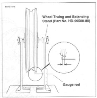
Figure 2-24. Checking Cast Rim Lateral Runout
