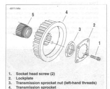
Figure 6-89. Transmission Sprocket
