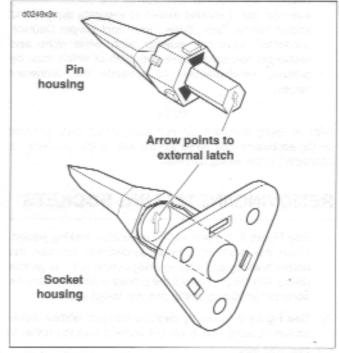
Figure B-9. Depress Terminal Latches/Back Out Plns
