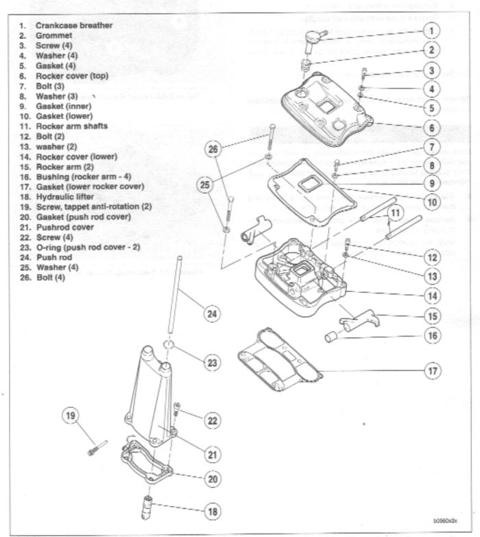
Figure 3-62. Rocker Arm and Pushrod Cover Assemblies
