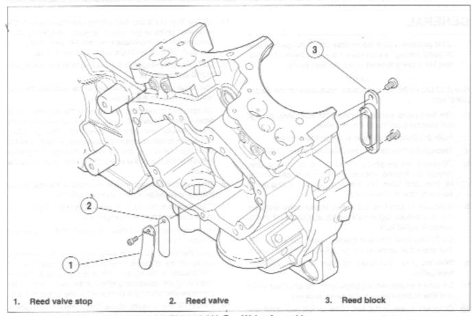
Figure 3-116. Reed Valve Assembly
