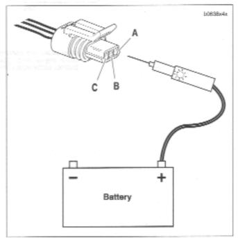
Figure 4-50. Testing IgnItlon Coll Connectors
