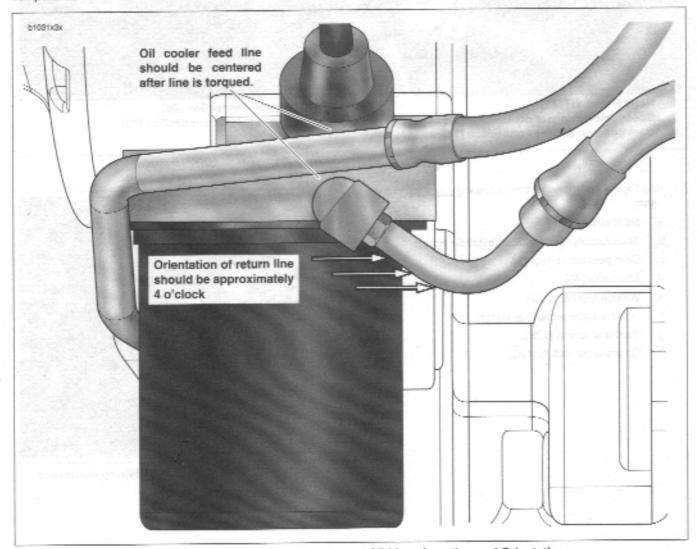
Figure 3-54. Oil Cooler Feed and Return Oll Lines Location and Orientation
