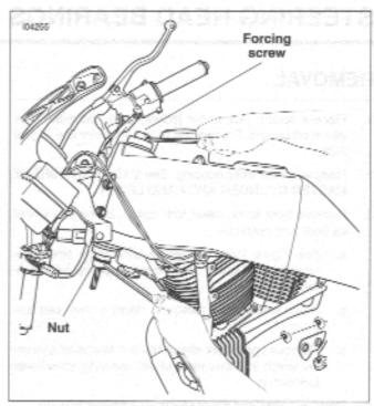
Figure 2-74. Install Bearings
