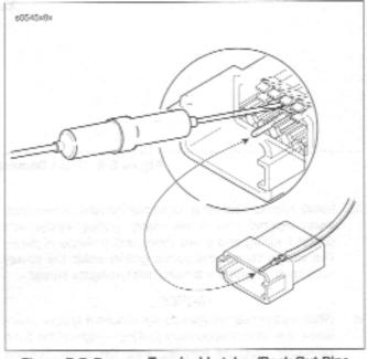
Figure B-7. Depress Terminal Latches/Back Out Pins
