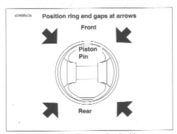
Figure 3-100. Ring End Gap Position
