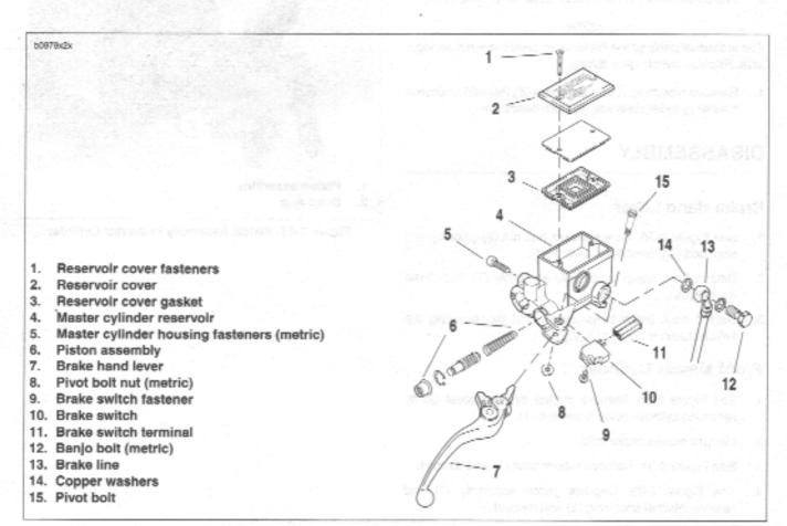
Figure 2-35. Front Brake Hand Lever Assembly
