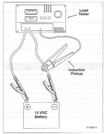
Figure 7-40. Load Test
