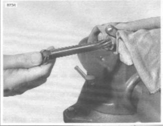
Figure 3-75. Replacing Rocker Arm Bushings
