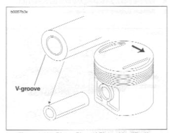
Figure 3-107. Piston Pin and Piston Identification
