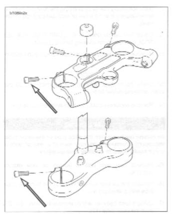
Figure 2-56. Upper and Lower Fork Clamp Pinch Fasteners
