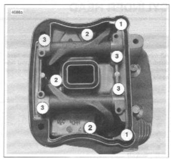
Figure 3-63. Lower Rocker Box Fasteners
