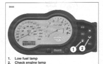
Figure 4-13. Check Engine Lamp
