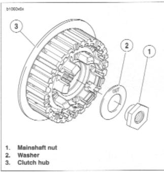
Figure 6-37. Mainshaft Nut and Washer
