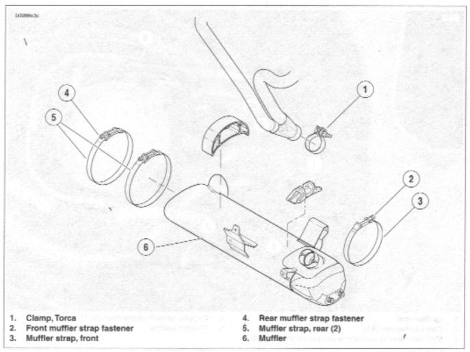
Figure 3-3. Muffler and Mounting System
