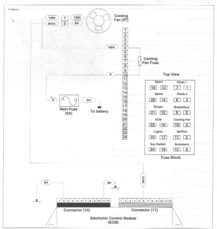
Figure 4-58. Cooling Fan Circuit
