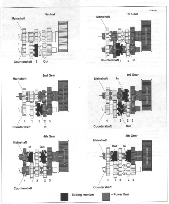
Figure 6-39. Transmission Power Flow
