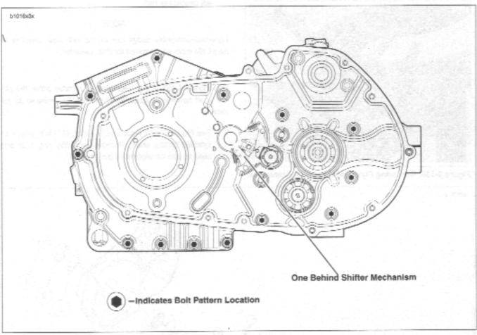
Figure 3-134. Crankcase Fasteners
