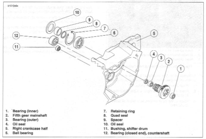
Figure 6-69. Transmission Assembly Right Crankcase Half
