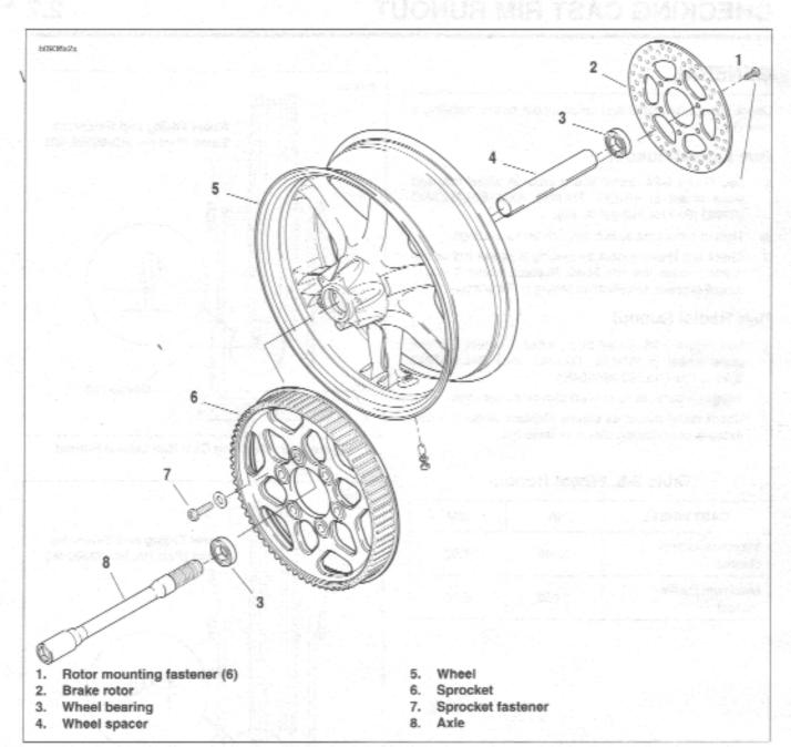
Figure 2-23. Rear Wheel Assembly
