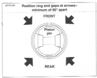
Figure 3-109, Ring End Gap Position
