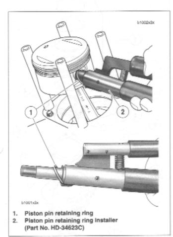
Figure 3-92. Removing Piston Pin Circlip
