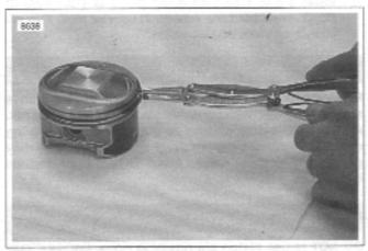
Figure 3-94. Removing Piston Rings
