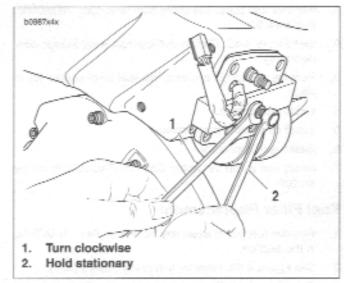
Figure 4-87. Fuel Pump Removal
