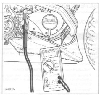
Figure 7-27. Check for Stator Resistance
