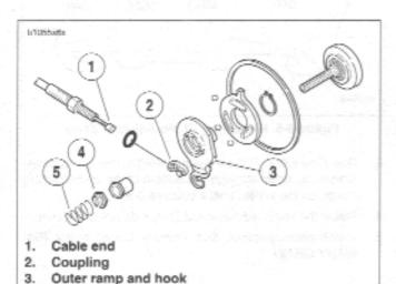
Figure 6-7. Clutch Release Mechanism
