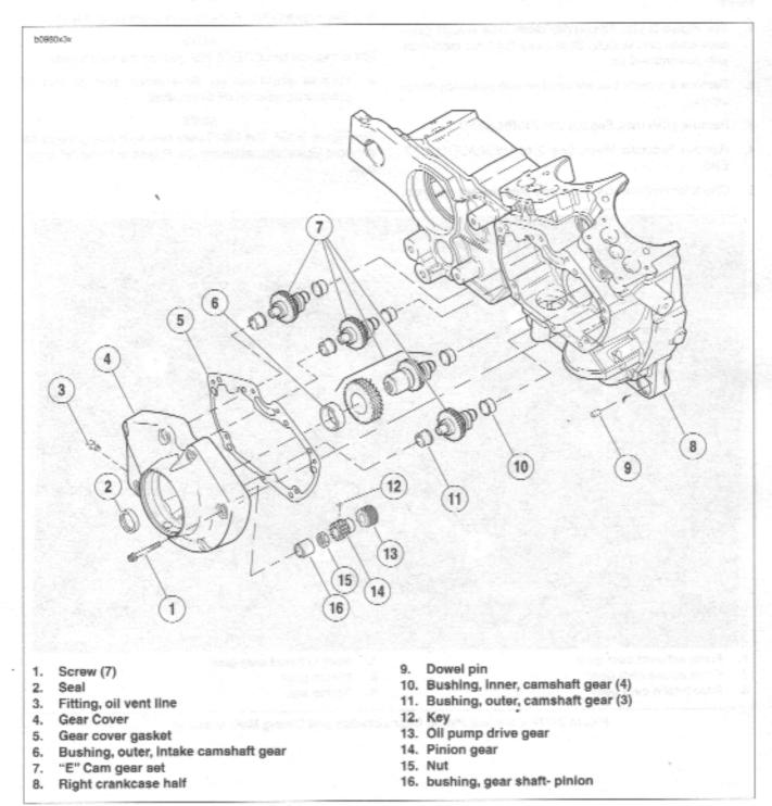
Figure 3-126, Gearcase Cover & Cam Assembly
