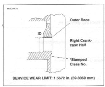
Figure 3-143. Factory Outer Race Sizes
