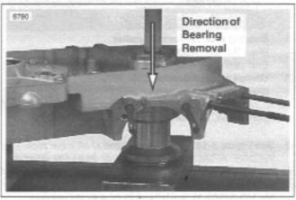
Figure 3-140. Removing Left Main Bearing from Crankcase
