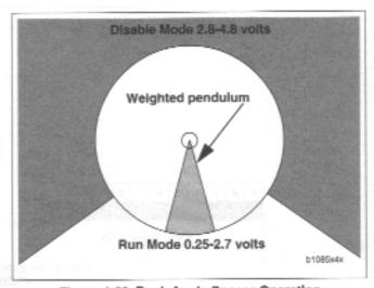
Figure 4-60. Bank Angle Sensor Operation
