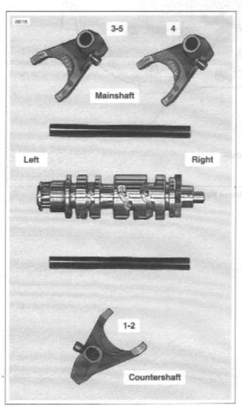
Figure 6-77. Shifter Forks, Drum and Shafts
