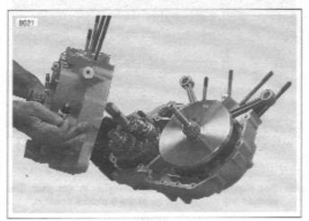
Figure 6-48. Separating Crankcase Halves
