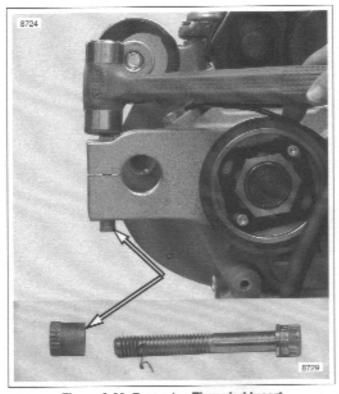
Figure 3-30. Removing Threaded Insert
