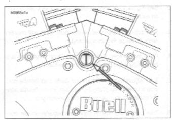
Figure 1-52. Correct Timing
