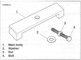
Figure 4-86. Fuel Pump Puller
