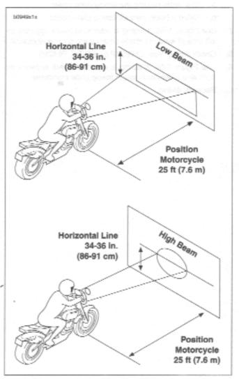
Figure 1-57. Checking Headlight Alignment
