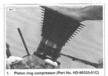
Figure 3-111. Compressing Piston Rings
