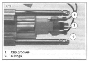
Figure 4-91. Regulator Housing O-rings
