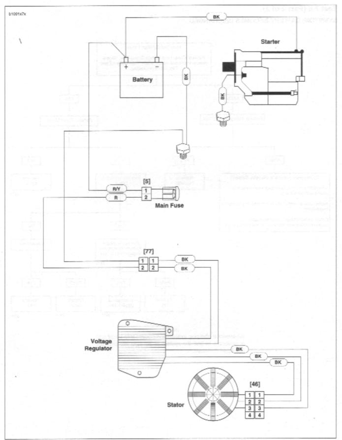
Figure 7-22. Charging System Circuit
