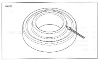
Figure 2-72. Steering Head Bearing Lip
