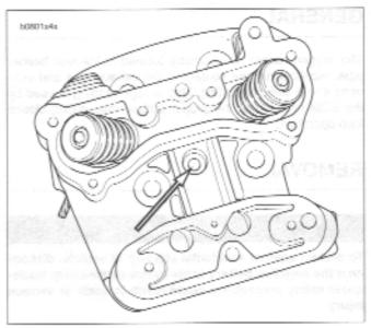
Figure 4-76. Englne Temperature Sensor Location (rear cylinder)
