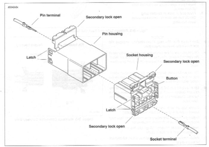
Figure B-1. 10-Place Amp Multilock Connector
