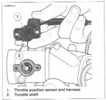
Figure 4-34. TP Sensor Assembly
