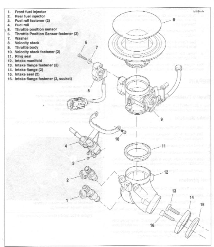
Figure 4-100. Throttle Body/Intake Manifold Assembly
