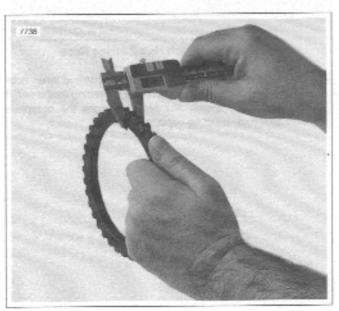
Figure 6-22. Measuring Friction Plates
