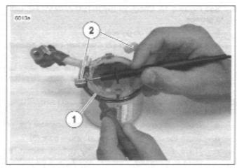
Figure 5-21. Grounded Field Test
