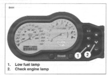
Figure 4-16. Check Engine Lamp
