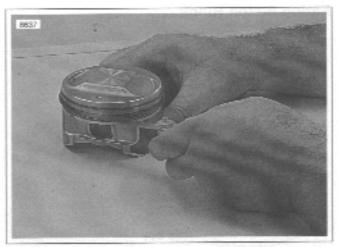
Figure 3-101. Measuring Ring Clearance in Groove
