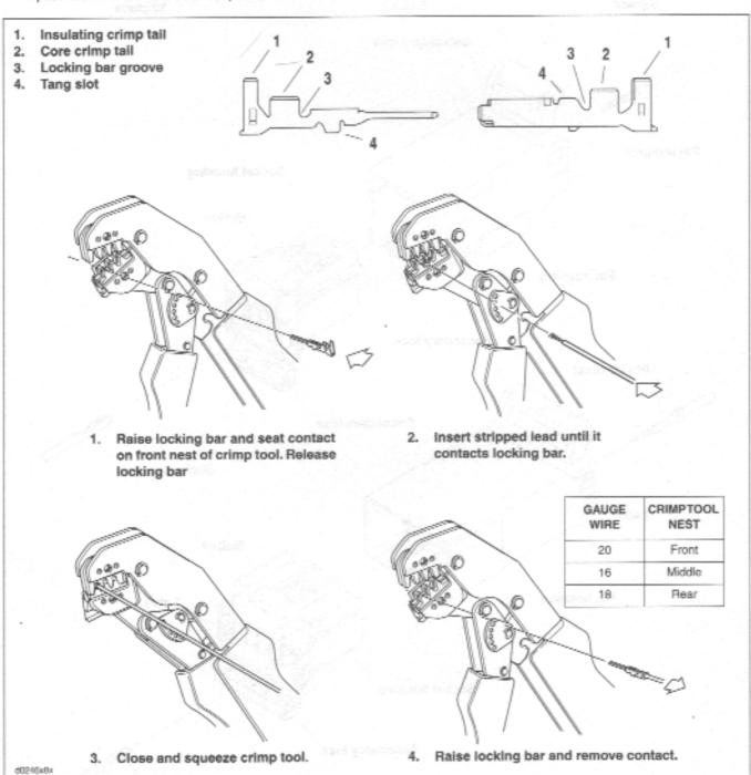
Figure B-5. Amp Multilock Crimping Procedure
