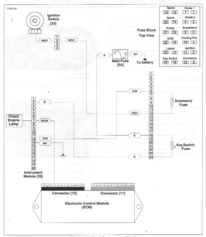
Figure 4-15. Check Engine Lamp Circuit
