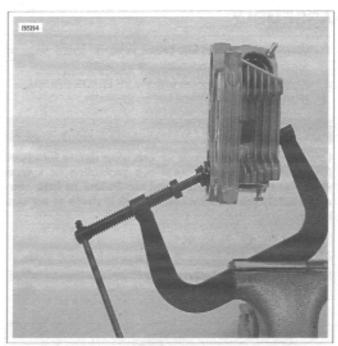
Figure 3-84. Valve Spring Compressor (Part No. HD-34736B)
