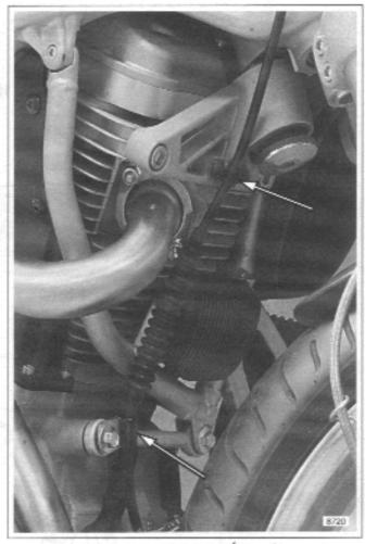
Figure 3-5. Clutch Cable Retaining Clamps
