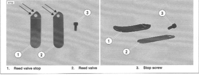
Figure 3-117. Reed Valve Stop and Reed Valve
