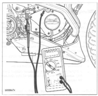
Figure 7-26. Test for Grounded Stator
