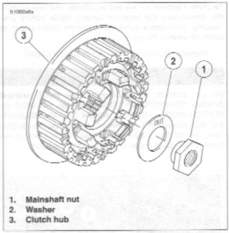
Figure 6-17. Malnshaft Nut and Washer
