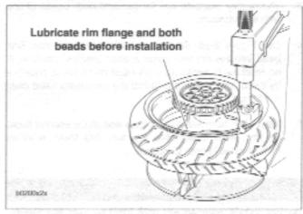
Figure 2-28. Starting Bead on Rim
