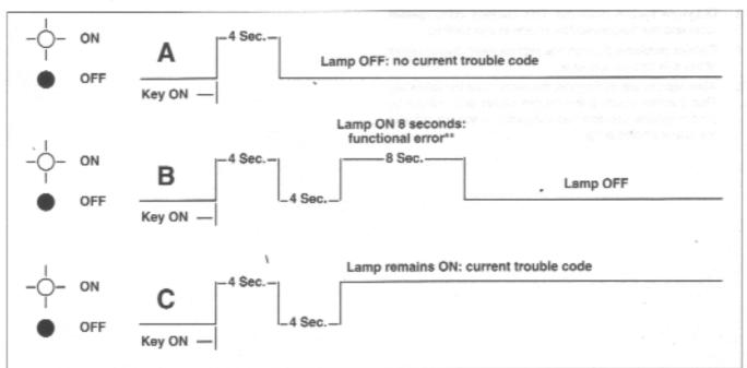
Figure 4-5. Check Englne Lamp Operation
