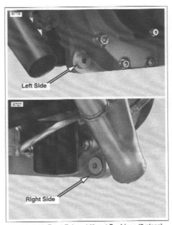
Figure 3-38. Front Exhaust Mount Bushings (2 piece)
