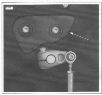
Figure 1-28. Primary Chain Inspection Cover
