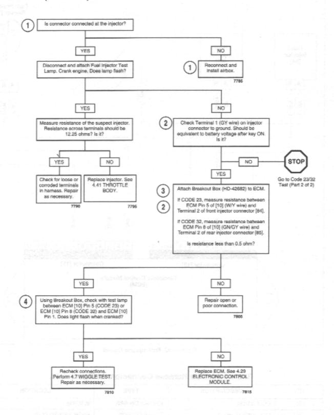
Clear codes and confirm proper operation with no check engine lamp. Codes can be cleared using DIGITAL TECHNICIAN (Part No. HD-44750).
