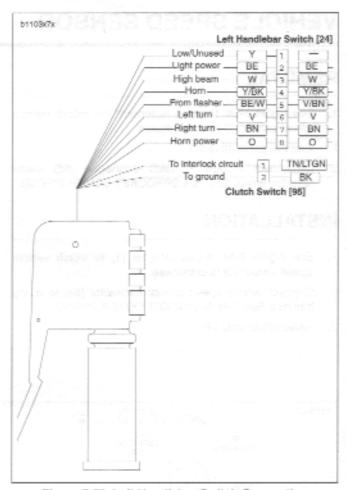
Figure 7-53. Left Handlebar Switch Connection
