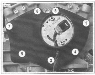
Figure 3-131. Gearcase Cover Mounting Screw Torque Sequence
