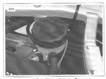
Figure 1-9. Rear Master Cylinder Reservoir
