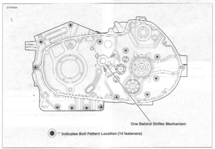
Figure 6-47. Crankcase Fasteners
