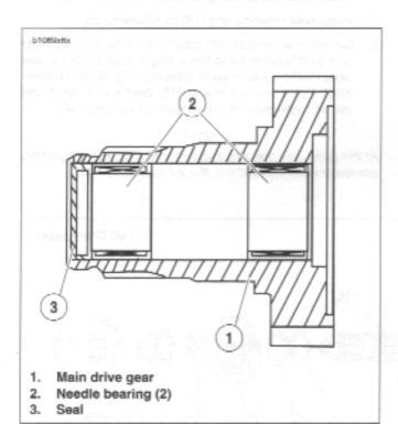
Figure 6-63. Main Drive Gear Assembly
