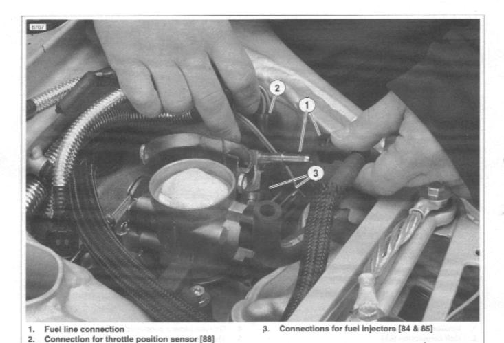
Figure 3-15. Fuel Line and DDFI Electrical Connections
