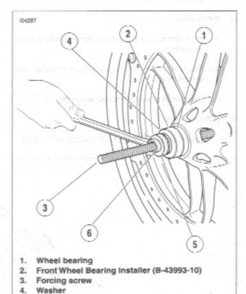
Figure 2-17. Install the Bearing
