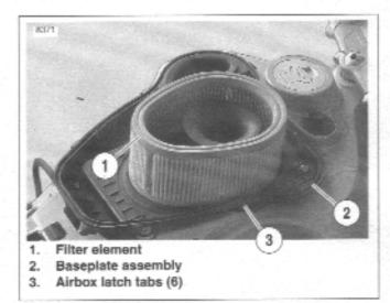
Figure 1-47. Installed Air Cleaner Filter Element
