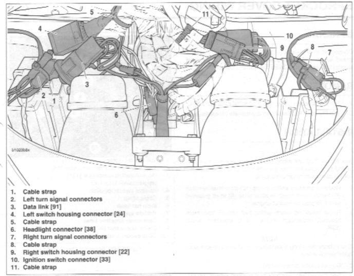
Figure 7-79. Fairing Wiring (viewed from underneath fairing)
