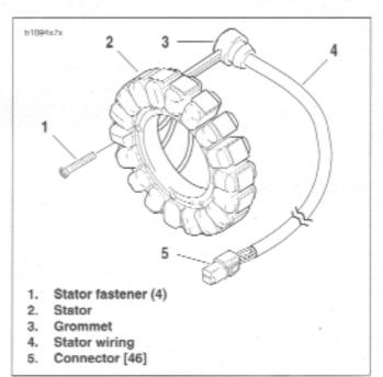
Figure 7-31. Stator Assembly
