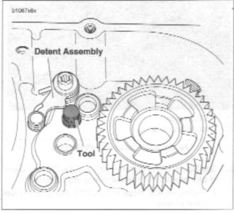
Figure 6-81. Gear Detent Assembly Ald (Part No. B-45520)
