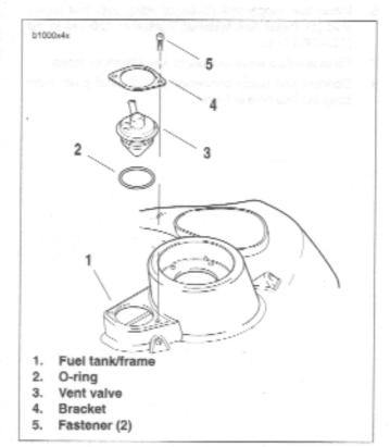
Figure 4-96. Fuel Tank Vent Valve
