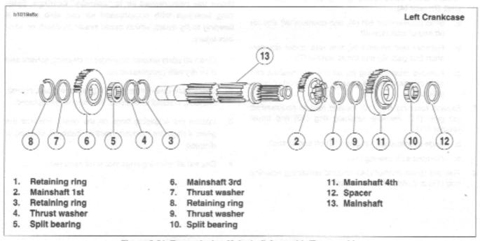
Figure 6-61. Transmission Mainshaft Assembly/Reassembly
