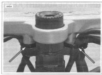
Figure 7-3. Cable Straps On Upper Fork Clamp
