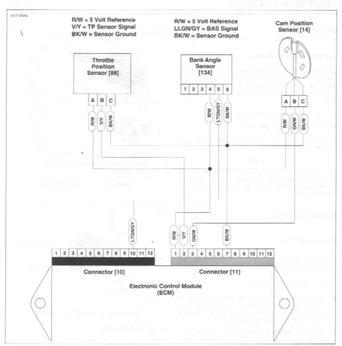
Figure 4-36. Throttle Position Sensor Circuit
