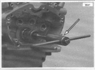
Figure 3-147. Lapping Pinion Shaft Main Bearing with Crankcase Main Bearing Lapping Tool (Part No. HD-96710-40B)
