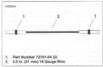
Figure 4-6. Diagnostic Test Wire
