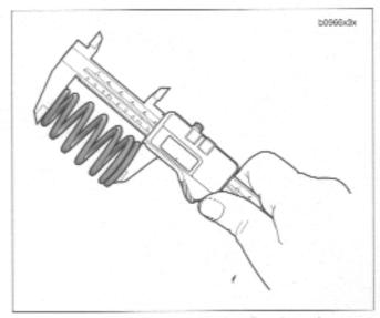
Figure 3-74. Checking Spring Free Length
