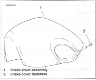
Figure 2-107. Intake Cover Assembly
