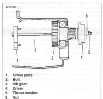
Figure 6-65. Removing Main Drive Gear
