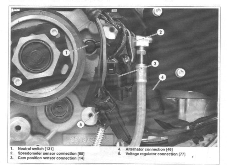
Figure 3-55. Electrical Connections
