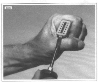
Figure B-6. Remove Secondary Locking Wedge
