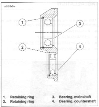
Figure 6-73. Ball Bearing Assembly
