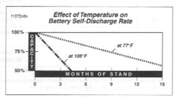
Figure 7-42. Battery Self-Discharge Rate
