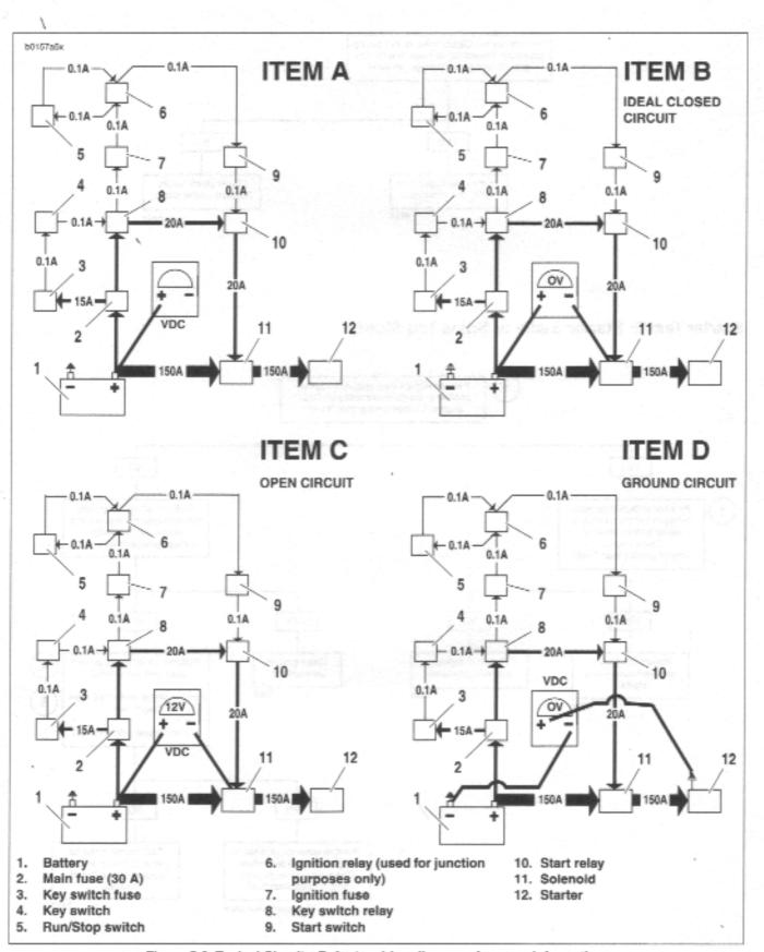
Figure 5-3. Typical Circuity. Refer to wiring diagrams for more Information.
