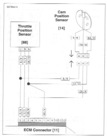
Figure 4-70. Connecting Sensor Wires
