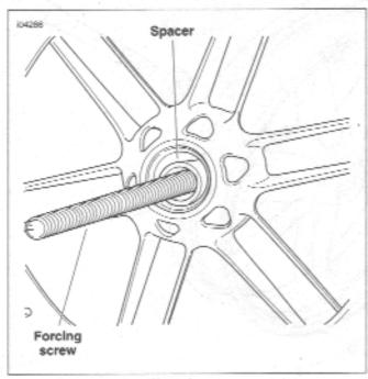
Figure 2-16. Install the Spacer
