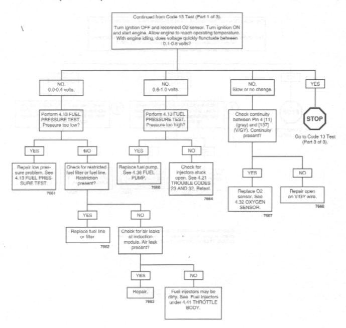
Clear codes and confirm proper operation with no check engine lamp. Codes can be cleared using DIGITAL TECHNICIAN (Part No. HD-44750).
