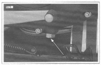
Figure 1-18. Primary Drain Plug
