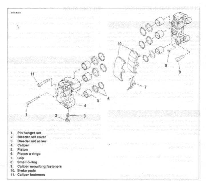
Figure 2-42. Front Caliper Assembly
