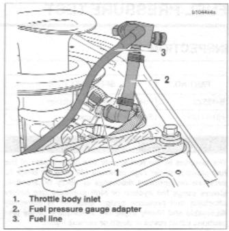
Figure 4-28. Fuel Pressure Gauge Adapter
