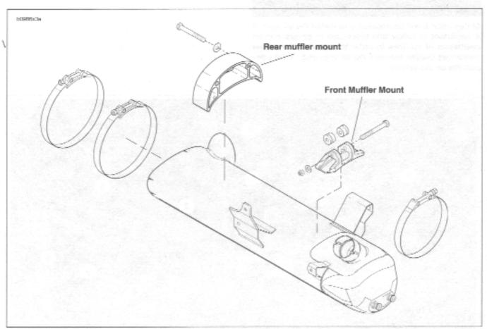
Figure 3-47. Muffler Mounting System
