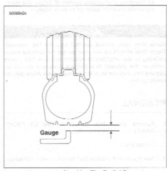
Figure 2-30. Checking Tire Radial Runout
