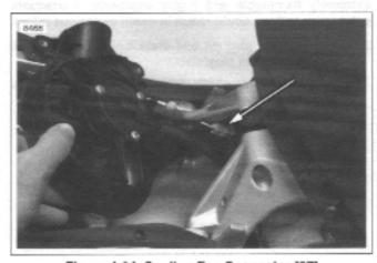
Figure 4-84. Cooling Fan Connector [97]
