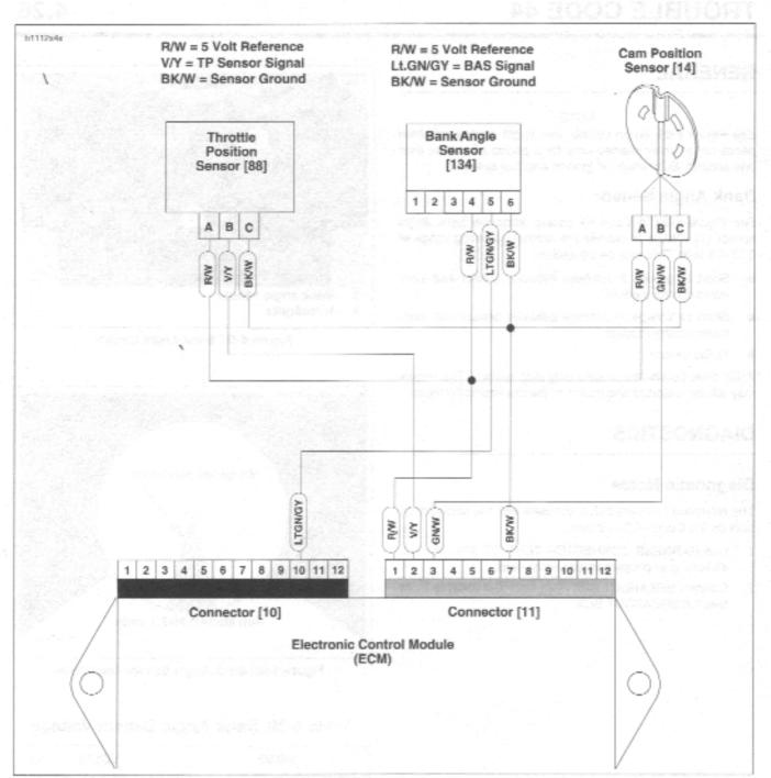
Figure 4-61. Bank Angle Sensor Circuit
