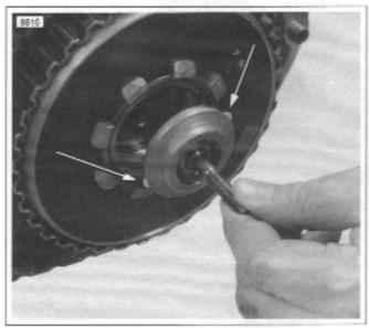
Figure 6-35. Adjusting Screw Assembly Aligning Tabs
