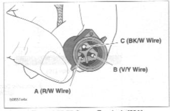
Figure 4-35. TP Sensor Terminals [88A]
