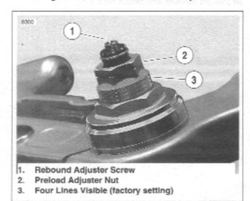
Figure 1-32. Front Fork Preload And Rebound Adjuster
