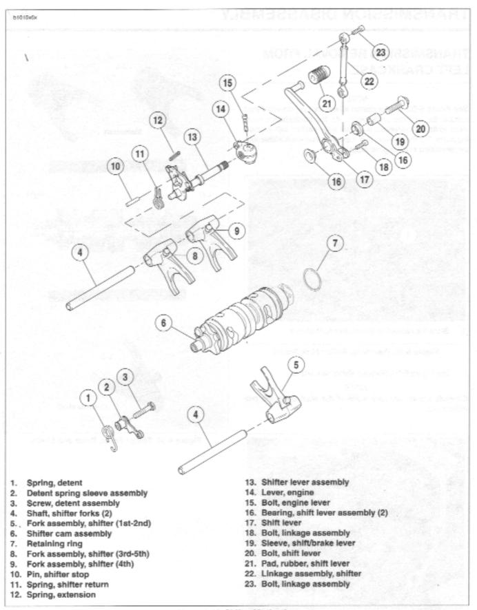
Figure 6-53. Shifter Mechanism
