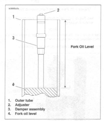
Figure 1-41. Measuring Fork Oil Level
