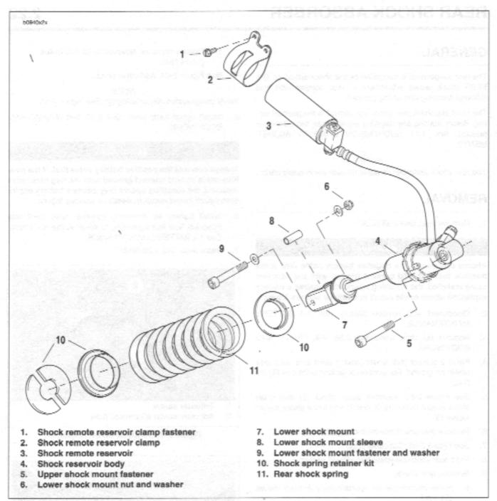
Figure 2-85. Rear Shock Absorber Assembly
