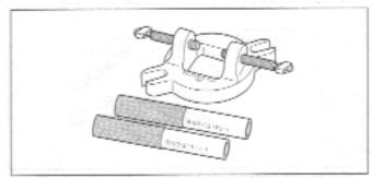
Part No. HD-95952-33B Connecting Rod Clamping Tool
