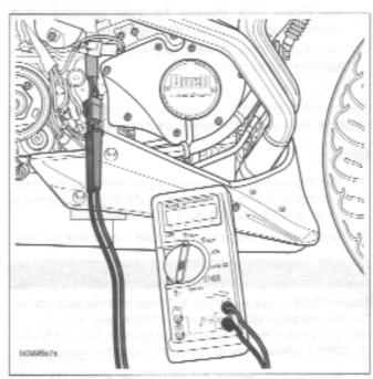
Figure 7-28. Check Stator AC Voltage Output
