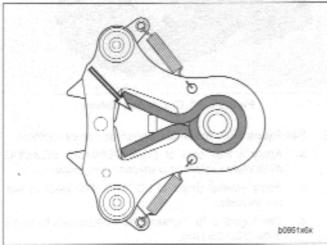
Figure 6-85. Shifter Shaft Return Spring (Incorrectly Installed)
