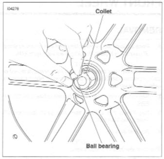
Figure 2-8. Install Collet and Ball Bearing
