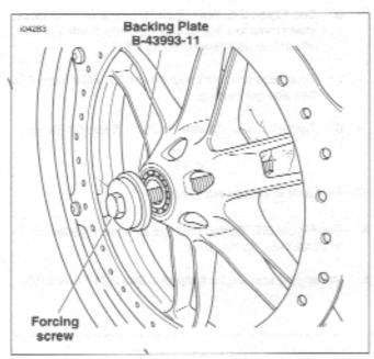
Figure 2-15. Insert Forcing Screw and Backing Plate
