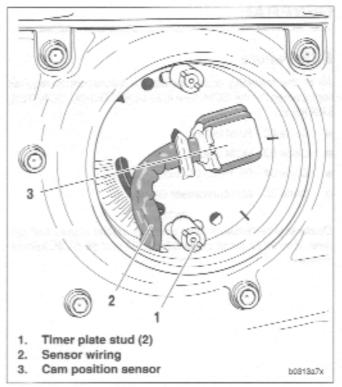
Figure 4-62. Cam Position Sensor
