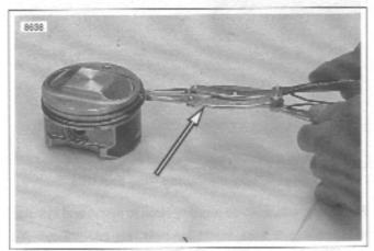
Figure 3-99. Installing Piston Rings Transmission Shaft Retaining Ring Pilers (Part No. J-5586)
