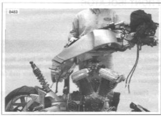
Figure 2-82. Lift Frame Off Motorcycle
