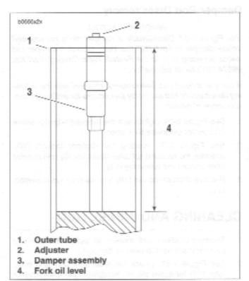
Figure 2-65. Measuring Fork Oil Level
