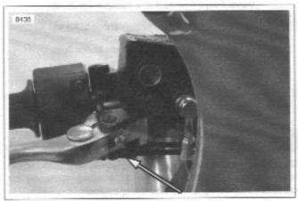
Figure 2-36. Brake Lamp Switch Connectors
