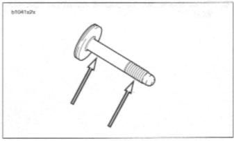
Figure 2-81, Lubrication Points on Front Isolator Bolt
