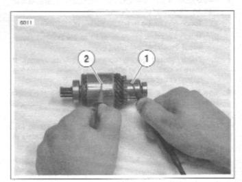
Figure 5-19. Grounded Armature Test
