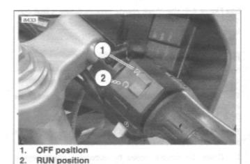
Figure 4-4. Engine Stop Switch
