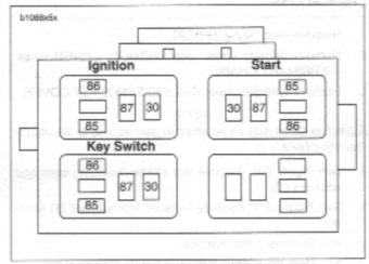
Figure 5-5. Relay Block (top view)
