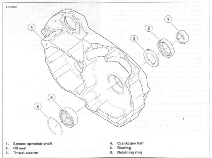
Figure 3-149. Left Main Bearing Assembly
