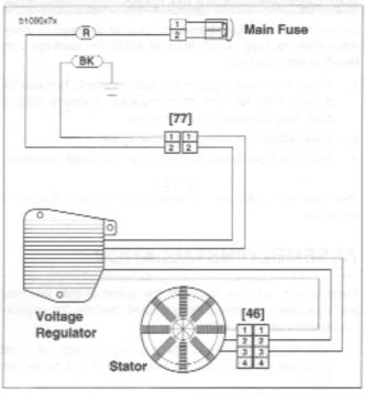
Figure 7-33. Voltage Regulator Connector [77]
