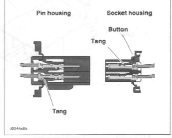
Figure B-3. Multilock Connector Cutaway View
