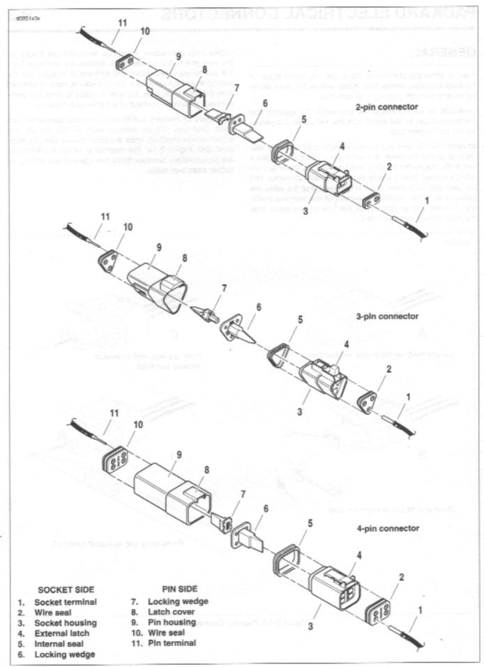
Figure B-13. 2-Pin, 3-pln and 4-pin Deutsch Connectors
