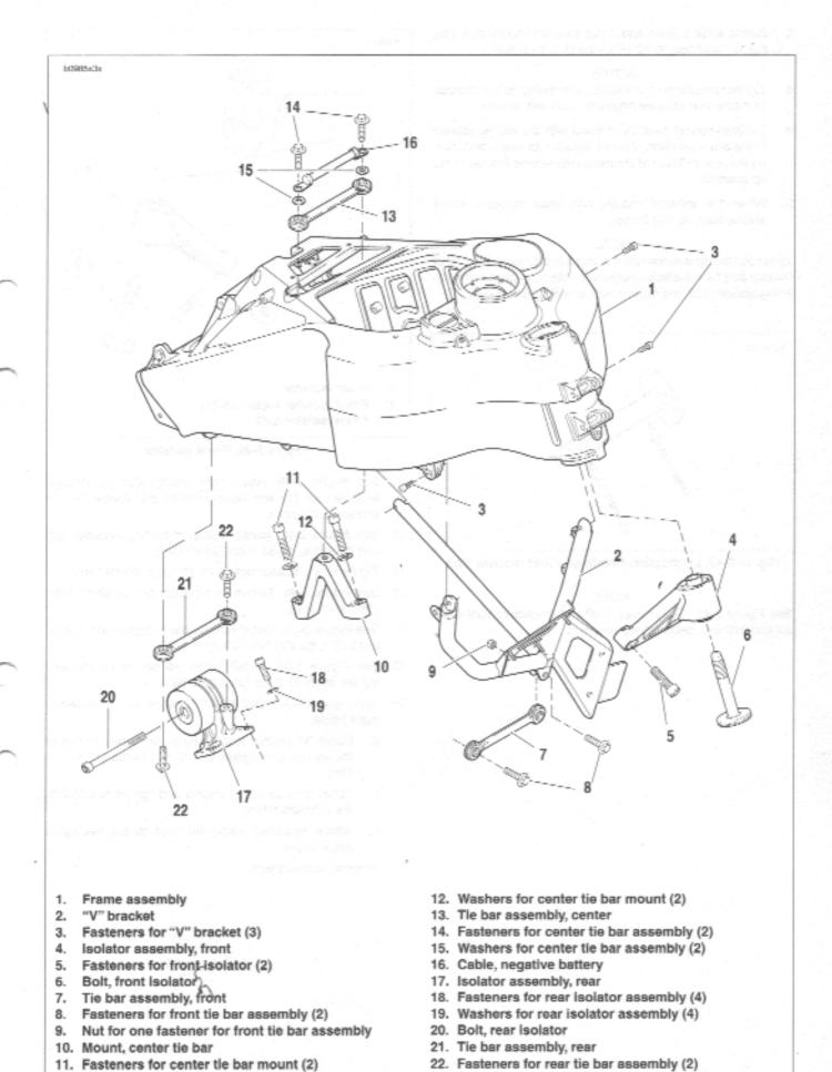
Figure 3-44. Engine Mounting System
