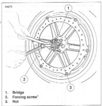
Figure 2-10. Remove the Bearing
