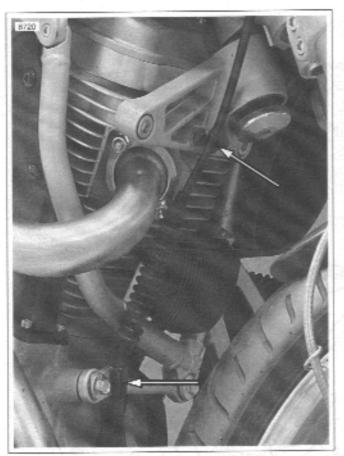
Figure 3-20. Clutch Cable Retaining Clamps
