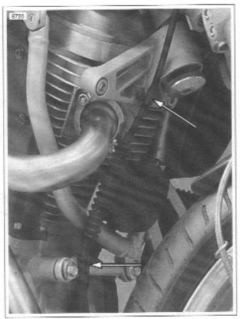
Figure 3-58. Clutch Cable Retaining Clamps
