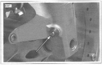
Figure 1-33. Front Fork Compression Damping Adjuster
