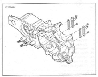
Figure 3-135. Piston Oil Jet Assemblies
