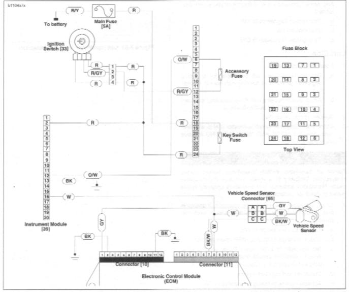
Figure 7-55. Vehicle Speed Sensor Wiring
