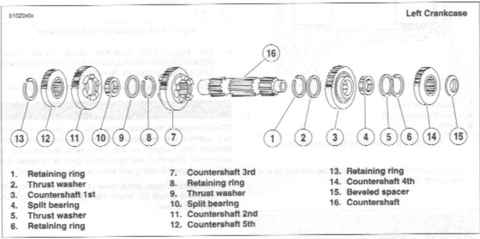
Figure 6-62. Transmission Countershaft Assembly/Reassembly
