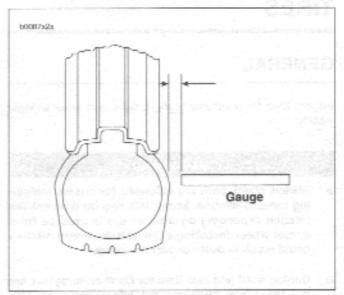
Figure 2-29. Checking Tire Lateral Runout
