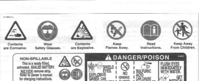
Figure 7-39. Battery Warning Label
