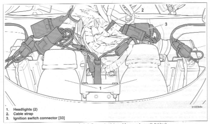
Figure 7-6, Ignition Switch Connector (viewed from underneath fairing)
