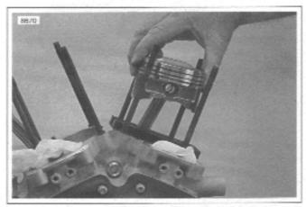
Figure 3-106. Piaton Support Plate (Part No. HD-42322)
