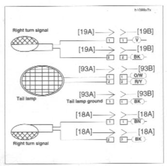
Figure 7-49. Rear Turn Signal Connections
