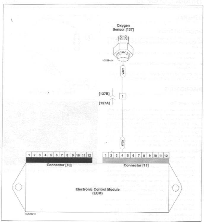
Figure 4-39. Oxygen Sensor Circuit
