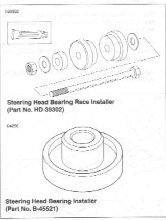
Figure 2-71. Steering Head Bearings Installation Tools
