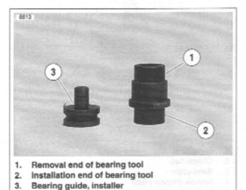
Figure 6-26. Clutch Shell Bearing Remover/Installer B-45926
