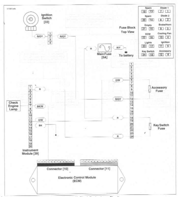
Figure 4-18. Check Engine Lamp Circuit
