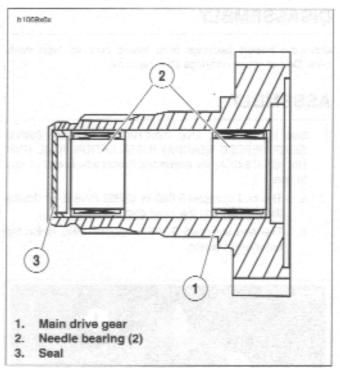
Figure 6-68. Main Drive Gear Assembly
