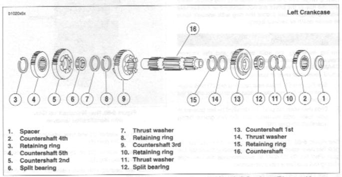
Figure 6-59, Transmission Countershaft Assembly Once Removed from Left Crankcase/Disassembly
