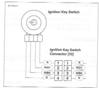
Figure 7-7. Ignition Key Switch Wiring
