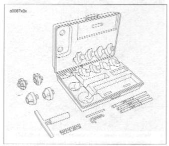
Figure 3-78. Neway Valve Seat Cutter
