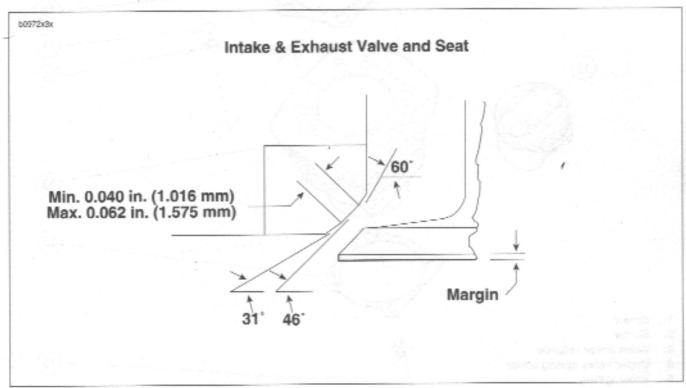
Figure 3-79, Valve and Seat Dimensions
