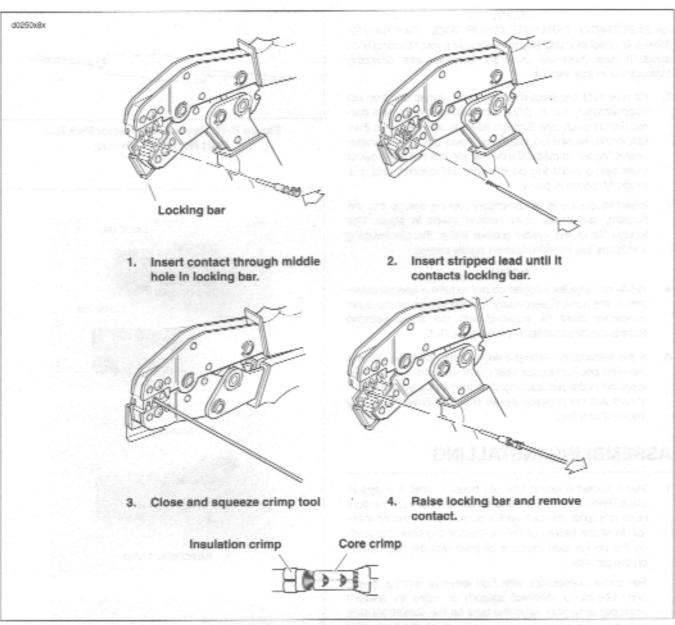
Figure B-12. Deutsch Crimping Procedure
