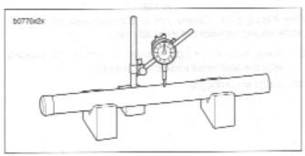
Figure 2-62. Pipe Runout
