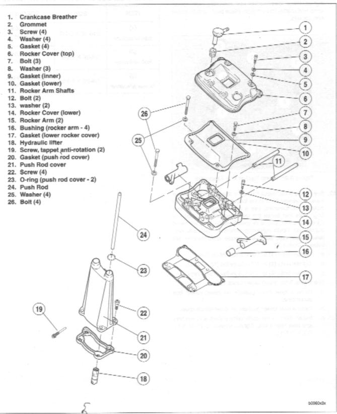
Figure 3-89. Rocker Arm and Pushrod Cover Assemblies
