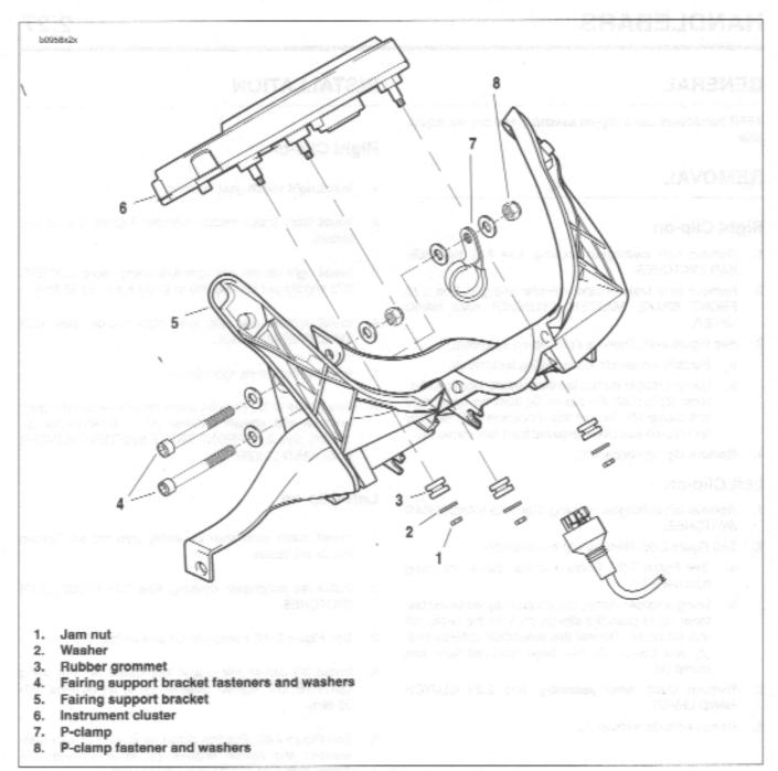
Figure 2-95. Fairing Support Bracket Assembly
