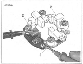
Figure 5-23. Brush Holder Insulation Test
