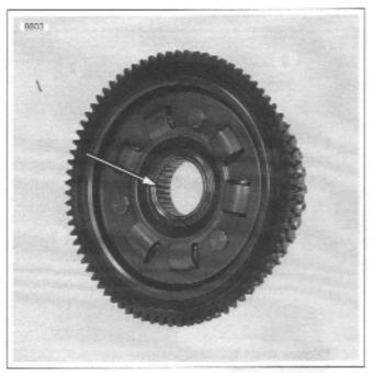
Figure 6-24. New Needle Bearing in Clutch Shell
