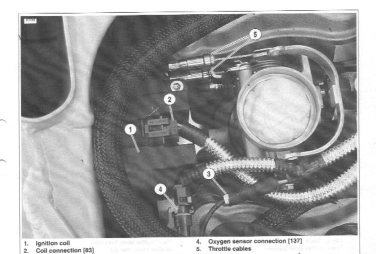
Figure 3-2. Electrical Connections and Throttle Cables
