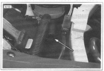
Figure 3-41. Transmission Vent Line
