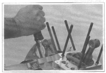
Figure 3-132. Checking Cam Gear End Play
