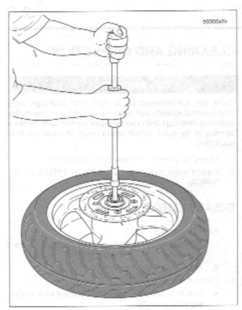
Figure 2-21. Removing Wheel Bearing
