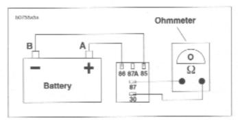
Figure 7-17. Starter Relay Test
