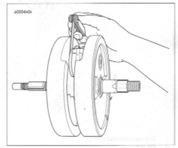
Figure 3-148. Checking Connecting Rod Side Play
