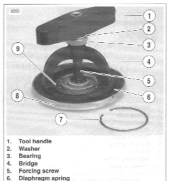
Figure 6-19. Pressure Plate Assembly
