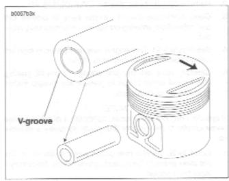
Figure 3-93. Piston Pln and Plston Identification
