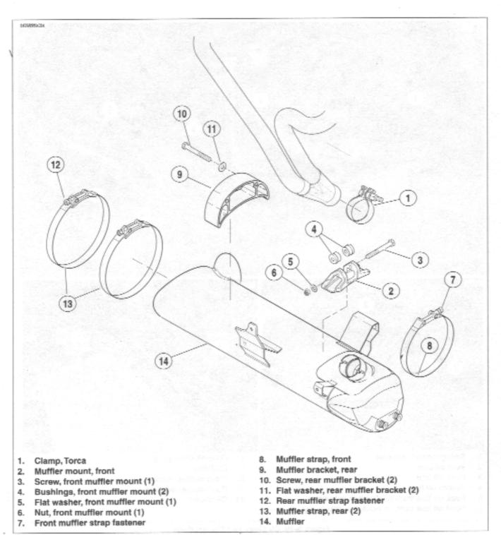
Figure 3-18. Muffler and Mounting System
