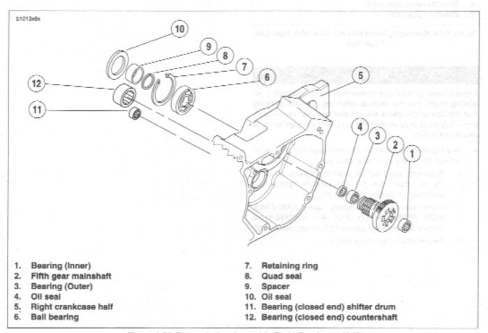
Figure 6-56. Transmission Assembly-Right Crankcase Half
