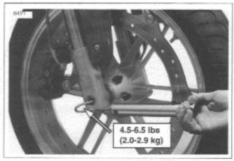
Figure 1-43. Measuring Steering Head Bearing Resistance
