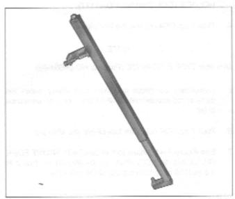
Figure 1-39. Fork Spring Compressing Tool
