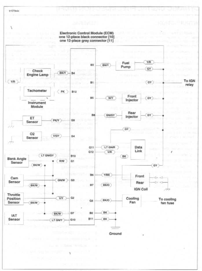
Figure 4-1. Buell Dynamic Digital Fuel Injection
