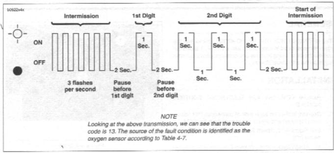
Figure 4-8. Check Engine Lamp Diagnostics
