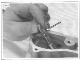
Figure 3-81. Valve Guide Seal Protector Sleeve
