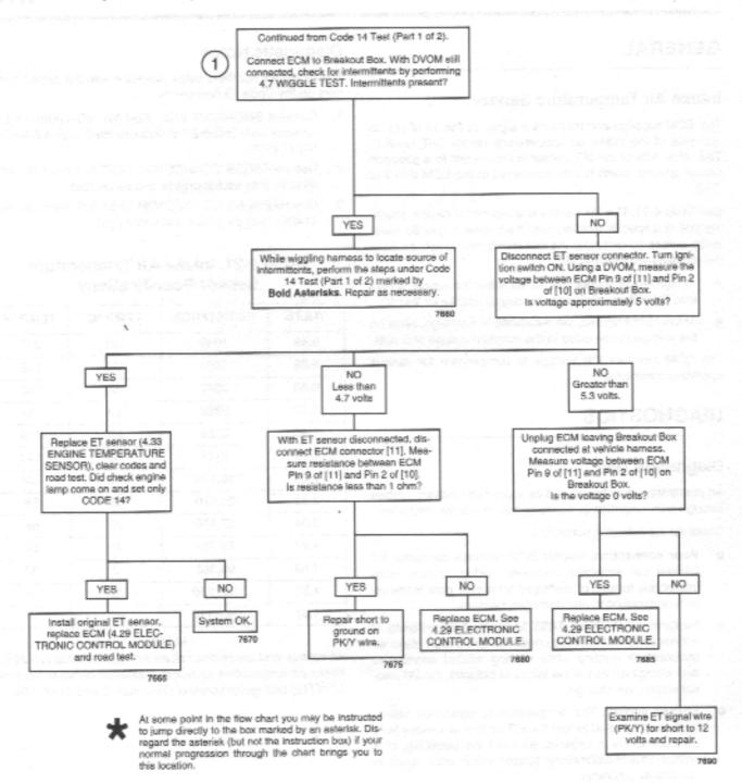
Clear codes and confirm proper operation with no check engine lamp. Codes can be cleared using DIGITAL TECHNICIAN (Part No. HD-44750).
