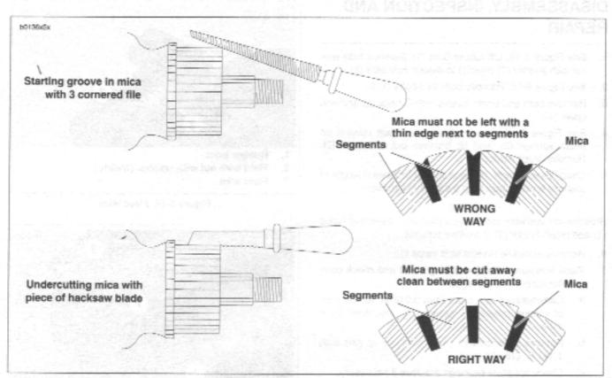
Figure 5-17. Undercutting Mica Separators
