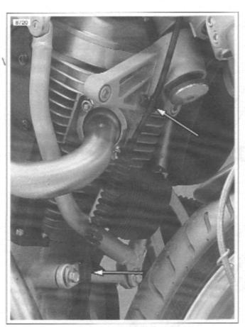
Figure 3-11. Clutch Cable Retaining Clamps
