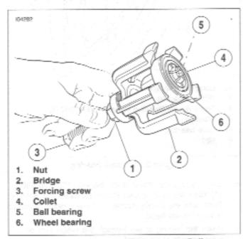
Figure 2-11. Removing Bearing from Puller
