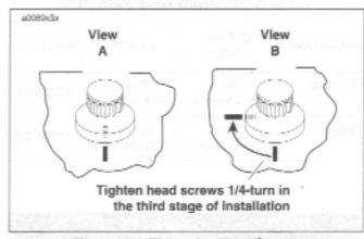
Figure 3-88. Tightening Head Screws
