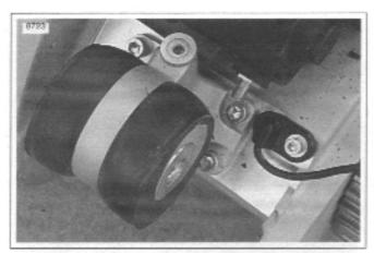
Figure 3-32. Rear Isolator and Mounting Hardware
