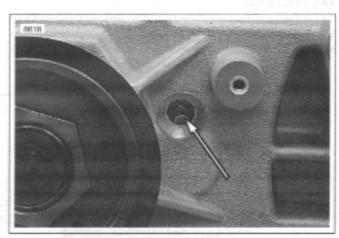
Figure 6-41. Shifter Drum Neutral Detent
