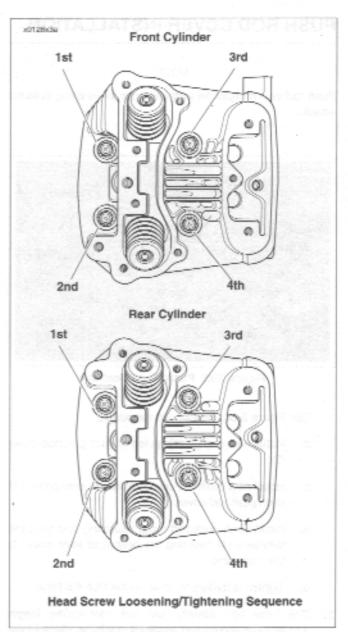
Figure 3-87. Head Screw Loosening/Tightening Sequence
