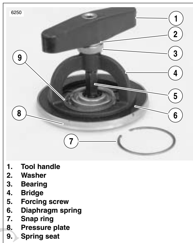
Figure 6-14. Pressure Plate Assembly
