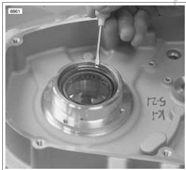
Figure 3-139. Sprocket Shaft Seal Retaining Ring
