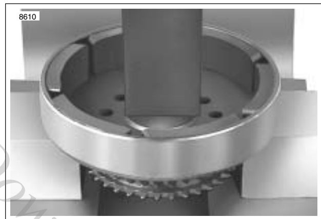
Figure 7-33. Removing Rotor From Sprocket
