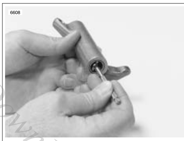
Figure 3-70. Measuring Rocker Arm Bushing Inner Diameter
