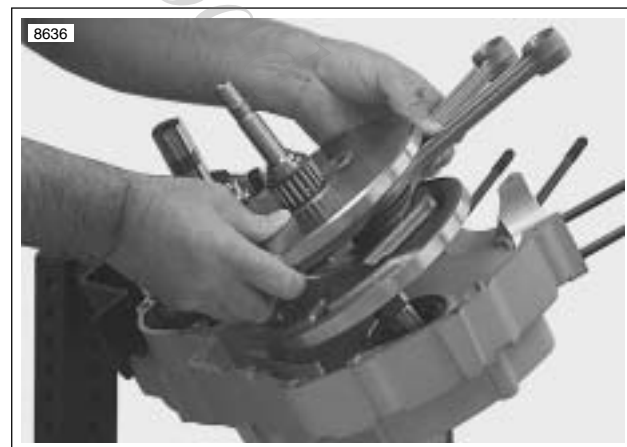
Figure 6-56. Removing Flywheels from Left Case Half
