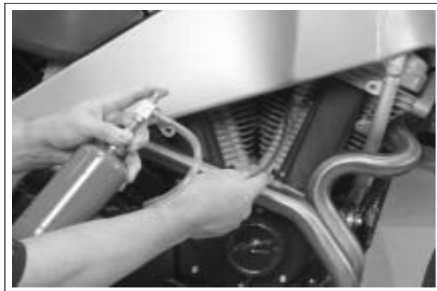
Figure 4-118. Checking for Intake Leak
