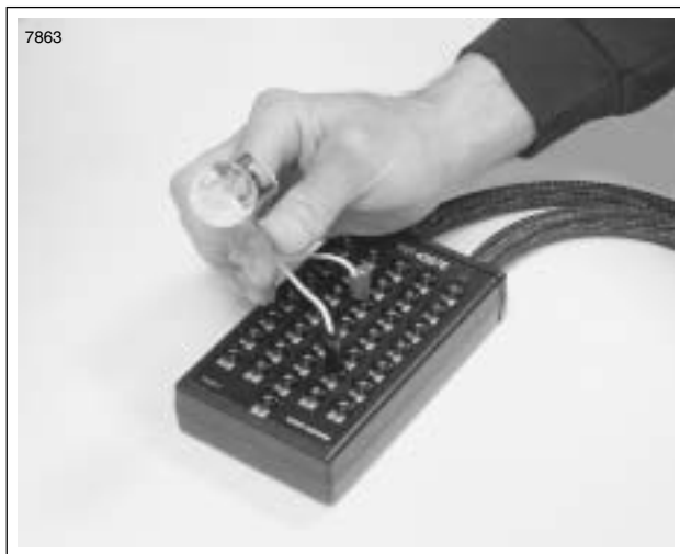
Figure 4-20. Ignition Coil Circuit Test
