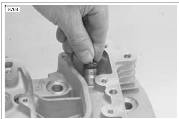
Figure 3-81. Valve Seal and Lower Collar Assembly Installation
