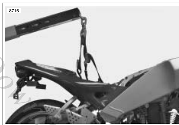
Figure 3-41. Supporting Vehicle for Assembly
