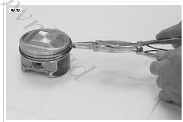
Figure 3-92. Removing Piston Rings
