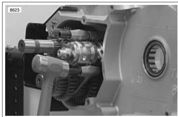
Figure 6-86. Installing Shift Fork Shafts
