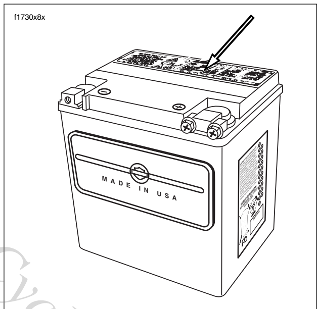
Figure 7-41. Battery Warning Label Location
