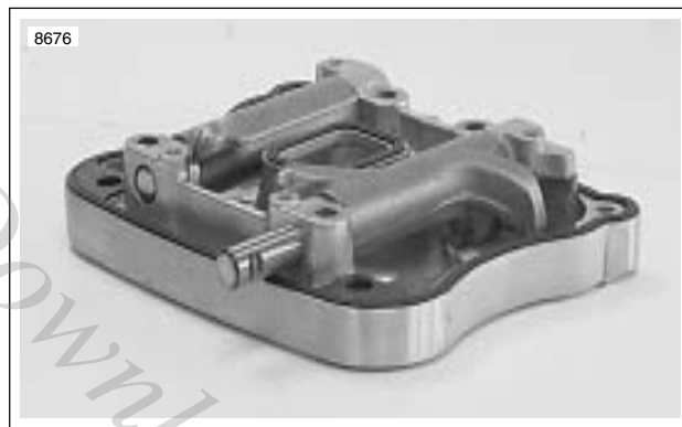
Figure 3-62. Removing Rocker Arm Shafts
