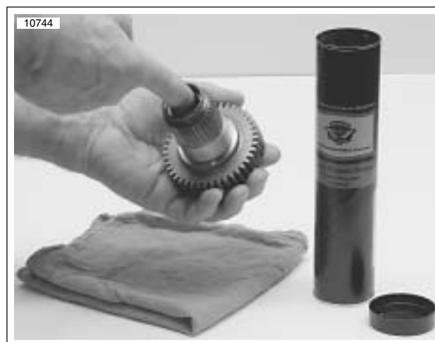
Figure 6-74. Lubricating Main Drive Gear Needle Bearings
