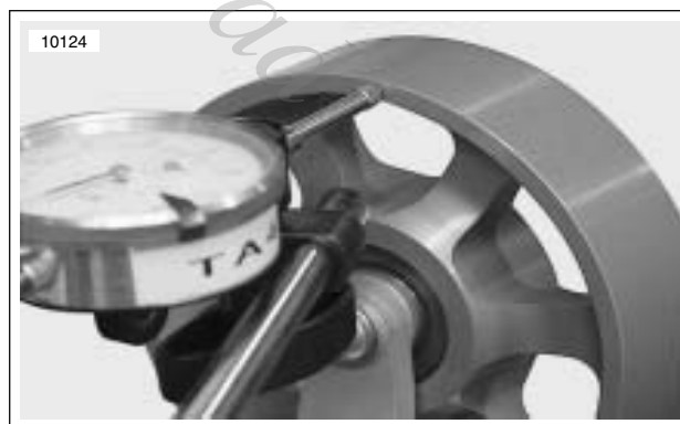
Figure 1-25. Checking Lateral Sideplay on Idler Pulley with a Dial Indicator
