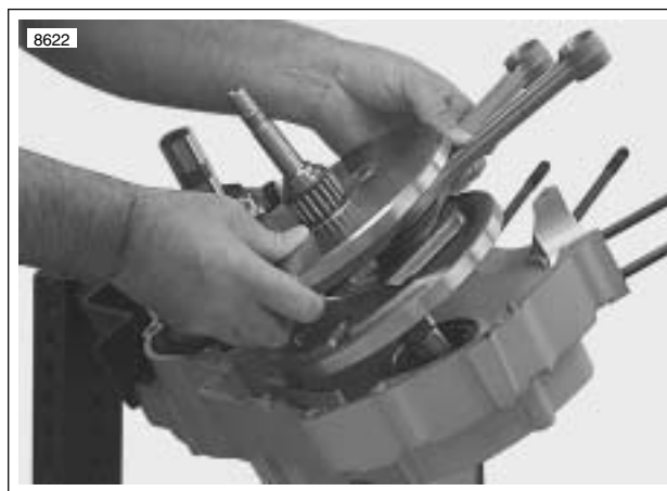
Figure 3-136. Removing Flywheels from Left Crankcase
