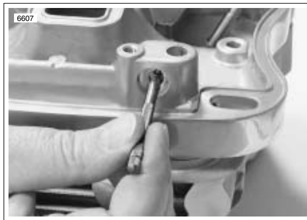
Figure 3-69. Measuring Rocker Arm Shaft Bore Diameter in Lower Rocker Cover
