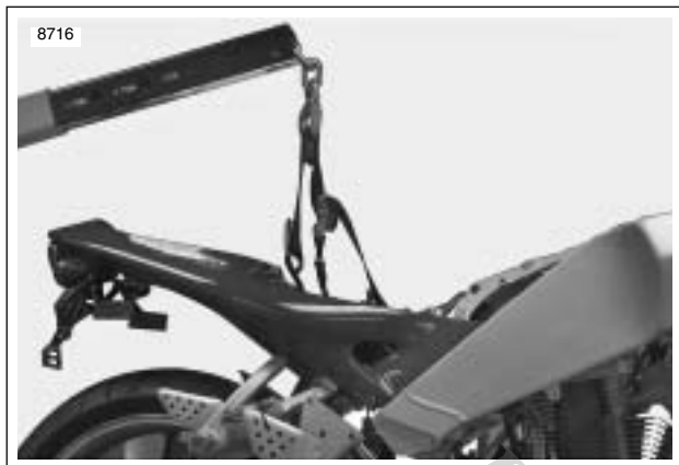
Figure 3-24. Supporting Vehicle for Disassembly
