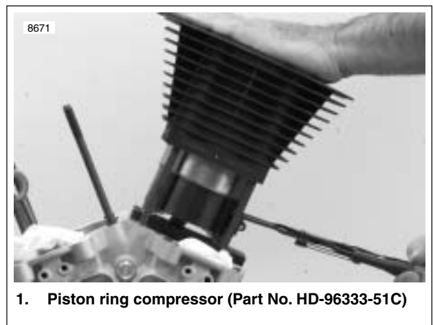
Figure 3-109. Compressing Piston Rings
