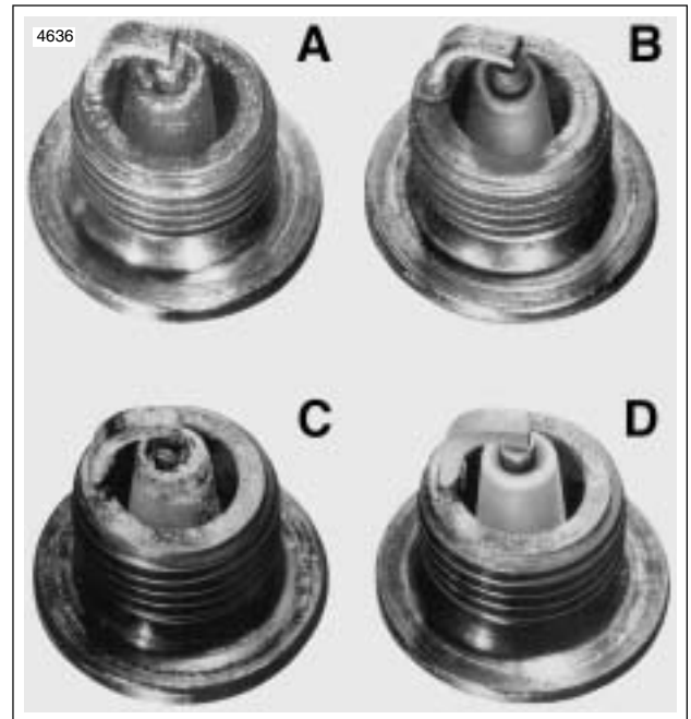
Figure 1-36. Typical Spark Plug Deposits
