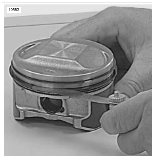
Figure 3-99. Measuring Ring Clearance in Groove
