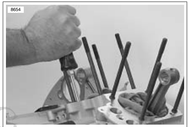
Figure 3-132. Checking Cam Gear End Play
