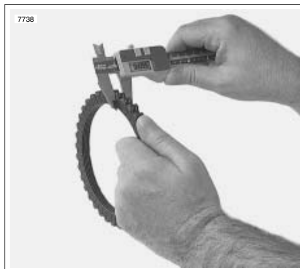
Figure 6-17. Measuring Friction Plates
