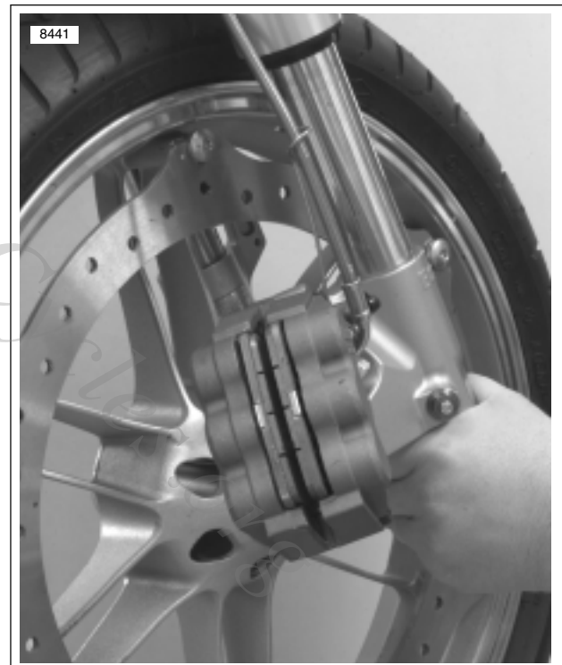
Figure 2-5. Front Wheel Removal
