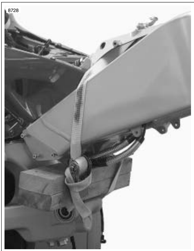
Figure 3-32. Securing Vehicle for Relocation (Typical)
