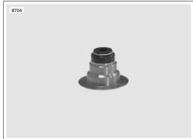
Figure 3-77. Valve Seal and Lower Collar Assembly (seal and lower collar replaced as assembly only)
