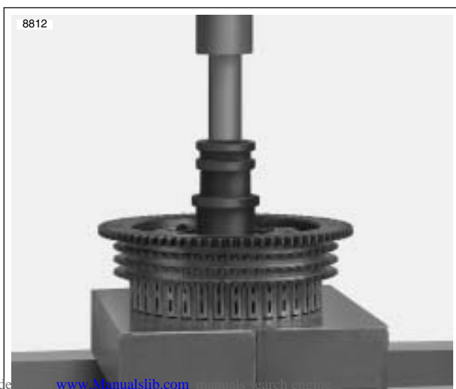
Figure 6-32. Installing Clutch Shell Needle Bearing Clutch Shell Bearing Remover/Installer (Part No. B-45926)
