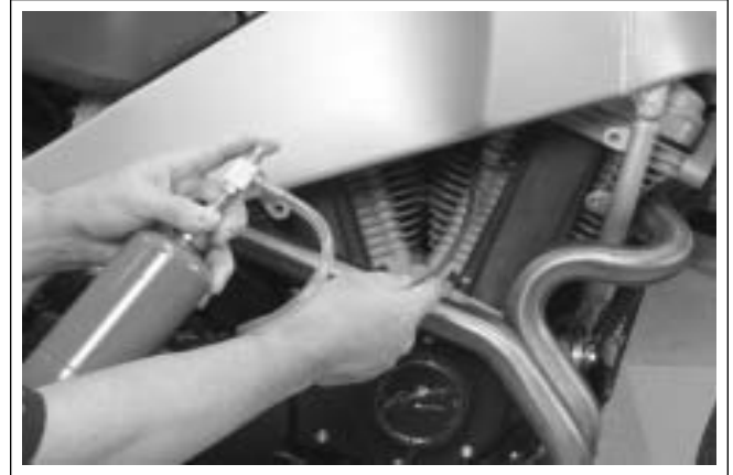
Figure 4-106. Checking for Intake Leak
