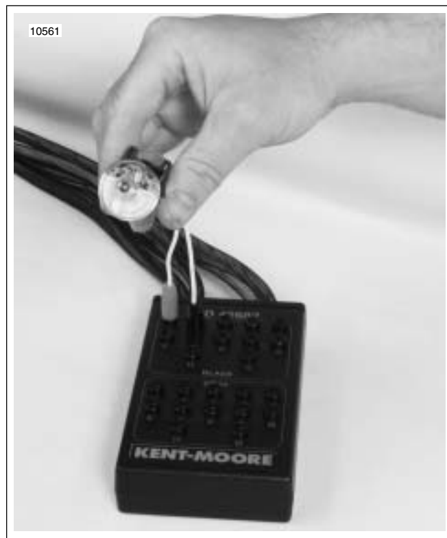
Figure 4-48. Testing Ignition Coil Connectors
