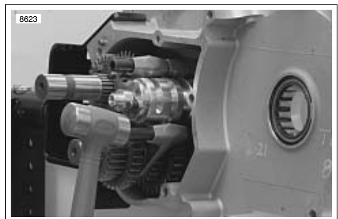
Figure 6-89. Installing Shift Fork Shafts
