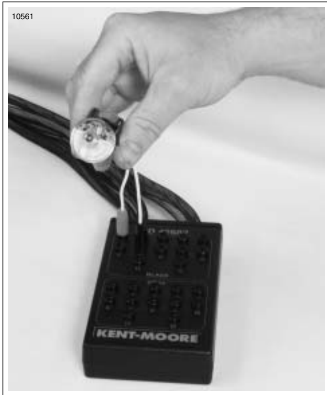
Figure 4-19. Ignition Coil Circuit Test
