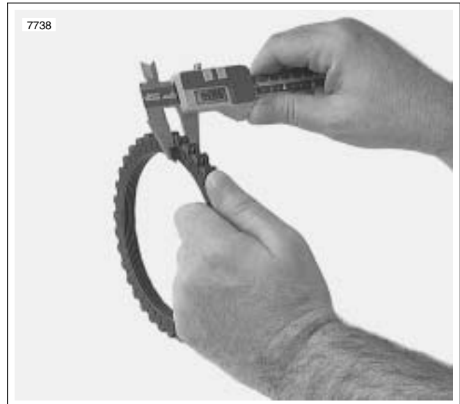
Figure 6-17. Measuring Friction Plates
