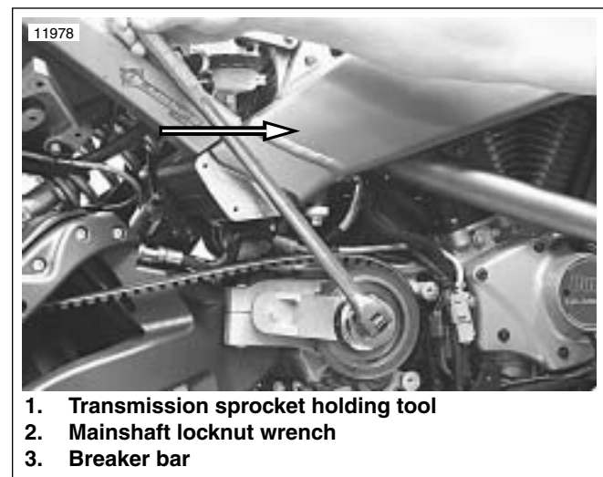
Figure 6-101. Removing Transmission Sprocket Locknut
