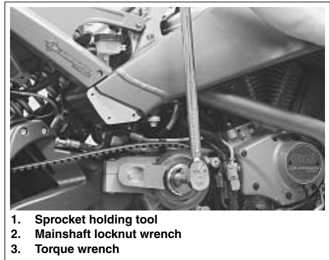
Figure 6-102. Transmission Sprocket Tightening
