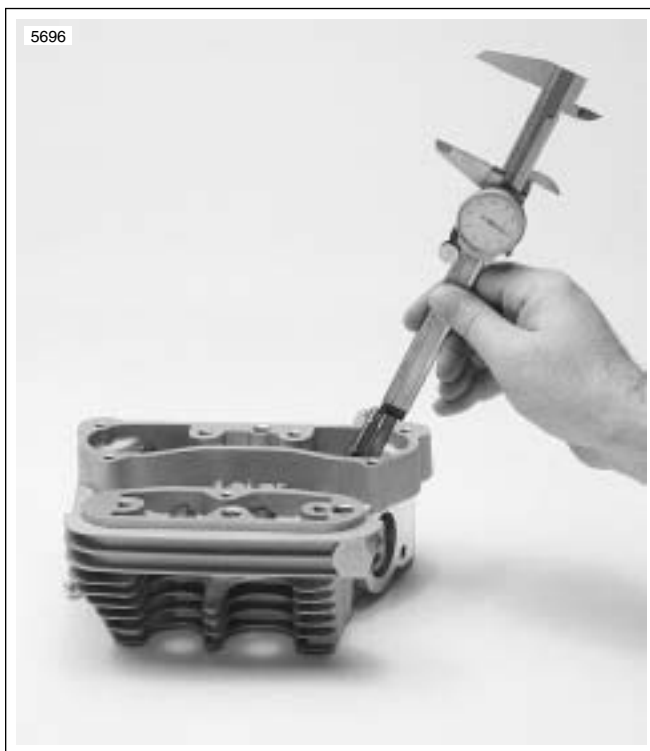
Figure 3-68. Measuring Valve Stem Protrusion
