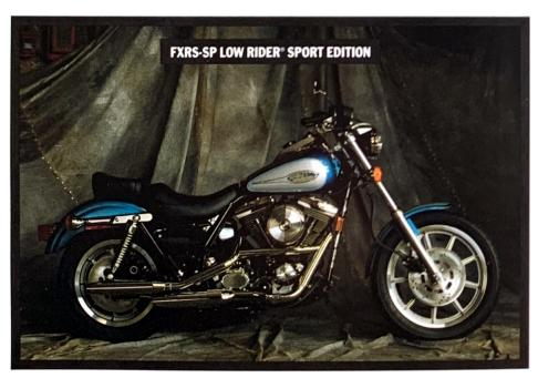
Evolution\* engine. Sport chassis. Triple disc brakes.
