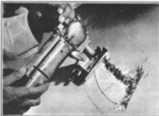
Figure 2J-7. Sawing Out Damaged Area
