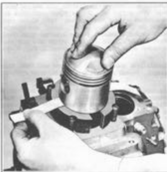
Figure 3C-11. Checking Rod Alignment
