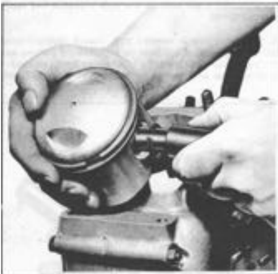
Figure 3C-14. Inserting Piston Pin Lock Ring
