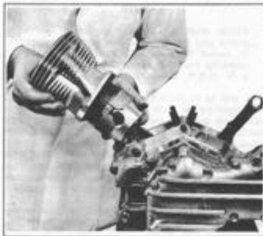
Figure 3C-15. Slipping Cylinder over Piston
