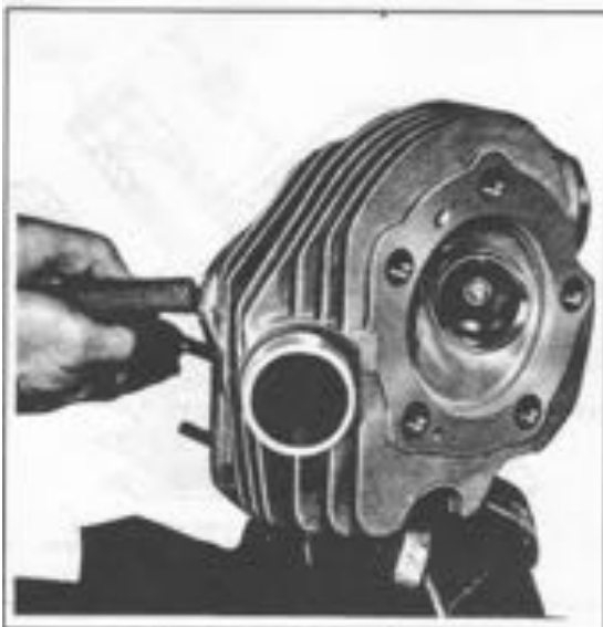
Figure 3B-4. Lapping Valves
