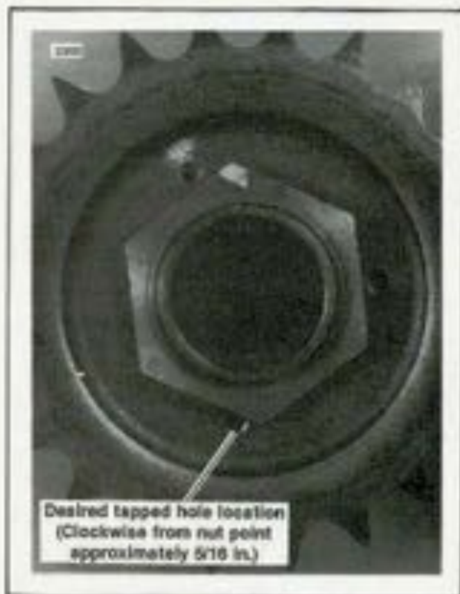
Figure 6-10. Securing Sprocket Nut
