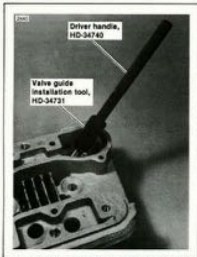
Figure 3-10. Installing Shoulder-less Valve Guides
