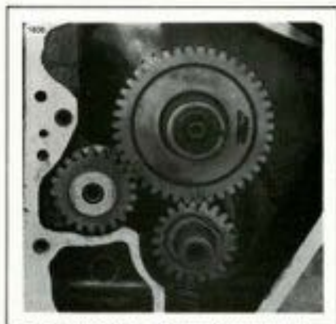
Figure 3-35. Timing Gears with Marks Aligned
