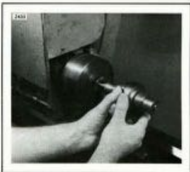
Figure 3-45. Lapping Connecting Rod
