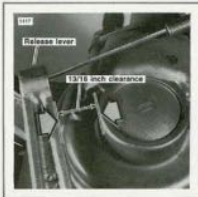
Figure 6-30. Release Lever Measurement
