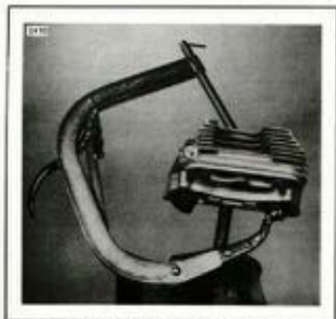
Figure 3-7. Compressing Valve Springs
