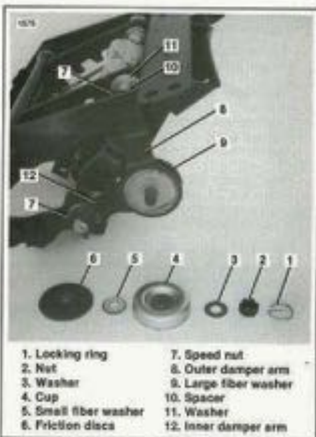
Figure 2-111. Friction Damper — 1981 and Later
