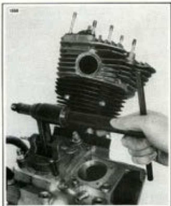
Figure 3-25. Replacing Rod Bushing
