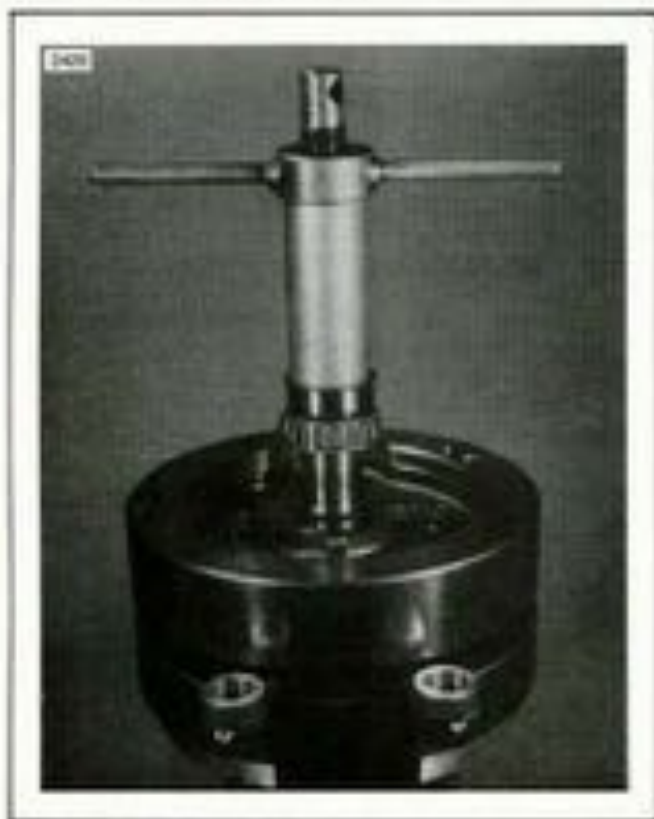
Figure 3-53. Pressing Bearing on Sprocket Shaft
