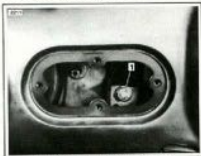
Figure 6-1. Primary Chain Adjustment
