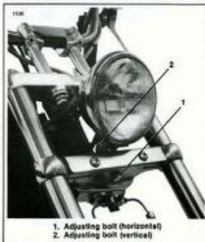
Figure 8-24. FXWG/FXDG/FXST Headlamp Adjustment
