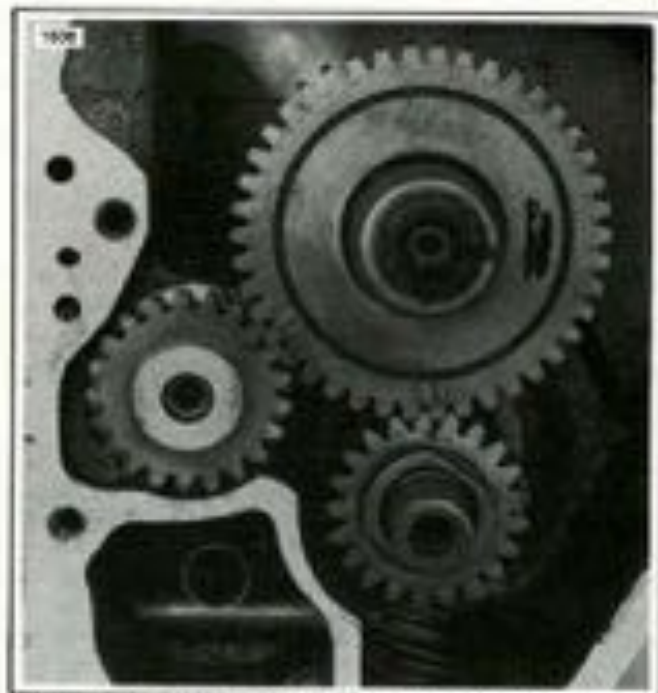
Figure 3-37. Timing Gears with Timing Marks Aligned
