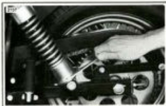
Figure 2-81. Adjusting Rear Shock Absorber
