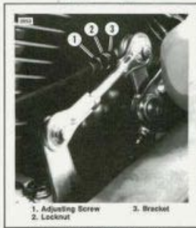
Figure 6-31. Clutch Cable Adjustment
