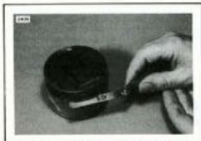
Figure 3-22. Measuring Ring Side Clearance
