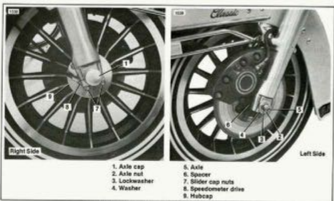
Figure 2-2. FL Front Wheel Mounting — 1981 and Later
