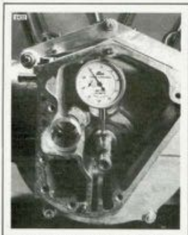
Figure 3-30. Checking Pinion Shaft Bearing
