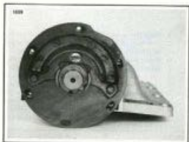
Figure 7-13. Aligning The Shifter Plate
