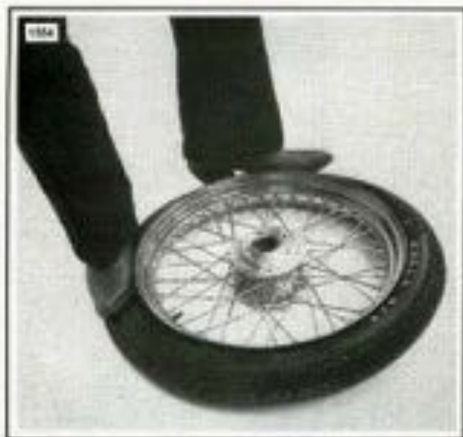
Figure 2-32. Loosening Tire Beads
