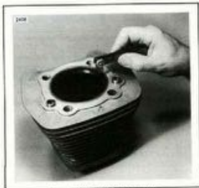
Figure 3-20. Checking Ring Gap
