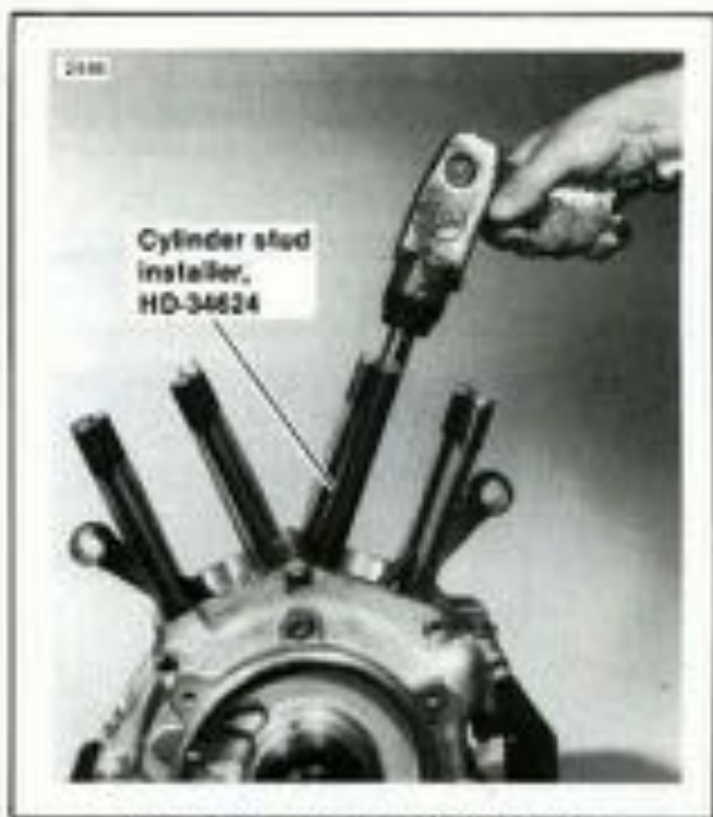
Figure 3-42. Installing Cylinder Studs
