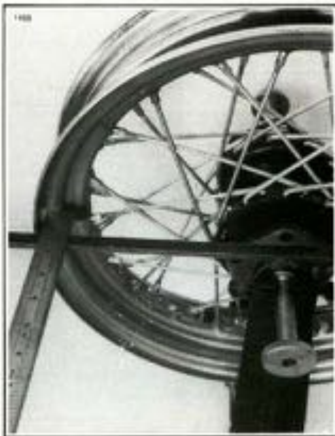
Figure 2-27. Centering 16 in. and 21 in. Hub
