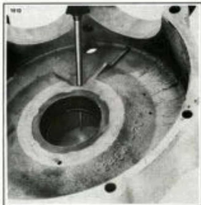
Figure 3-47. Removing Lock Ring
