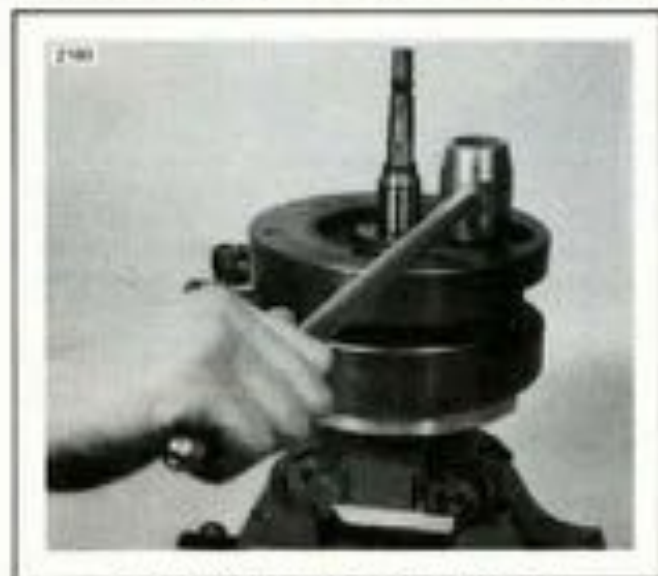
Figure 3-45. Removing Crank Pin Nut
