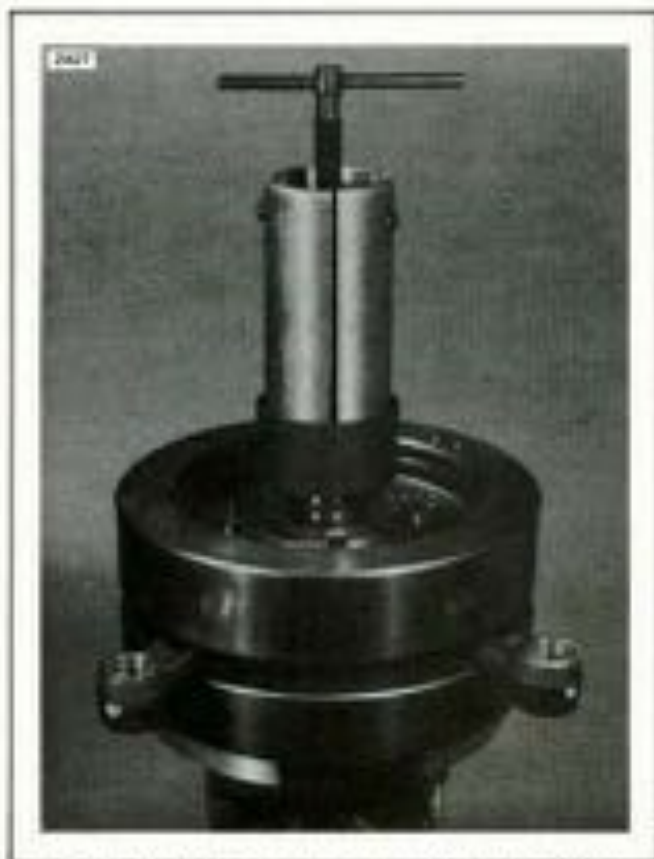
Figure 3-44. Pulling Bearing from Sprocket Shaft
