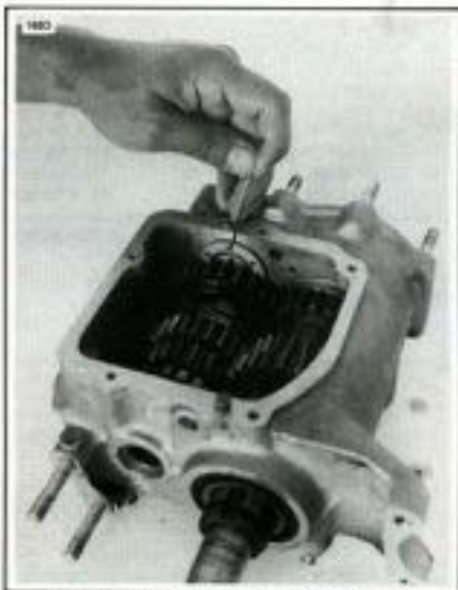
Figure 7-38. Removing Countershaft Washer
