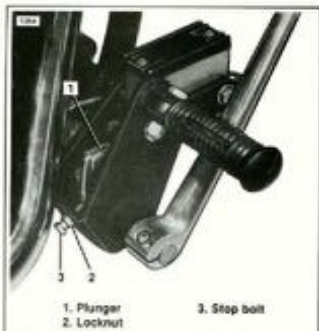
Figure 2-43. Rear Brake Pedal Adjustment 1983 & Earlier FXWG Only
