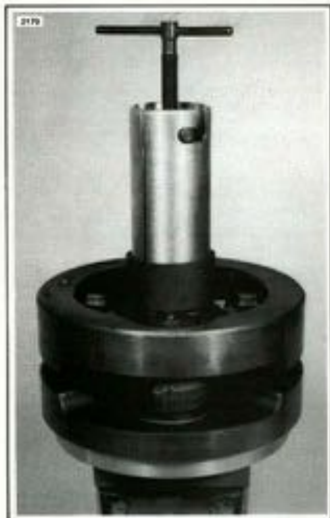
Figure 3-48. Pulling Bearing from Sprocket Shaft
