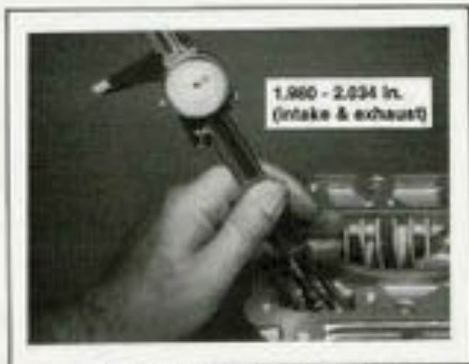
Figure 3-12. Valve Stem Protrusion
