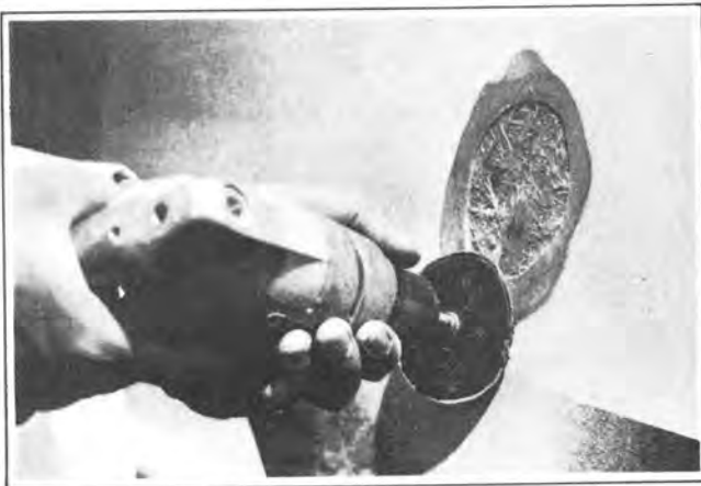
Figure 4-12. Rough Sanding Outside Surface
