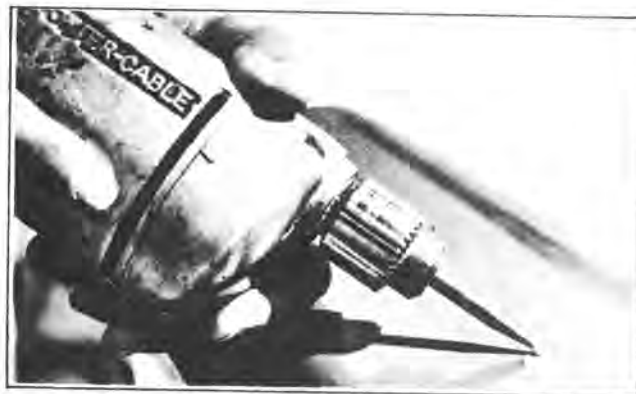
Figure 4-1. Roughing Damaged Area
