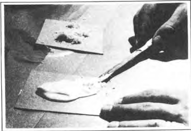
Figure 4-2. Mixing Gel Coat Glass Fibers
