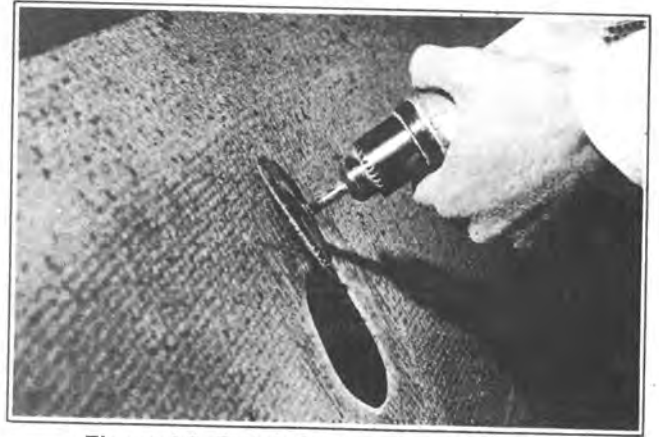
Figure 4-8. Rough Sanding Inside Surface
