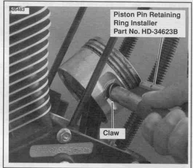
Figure 3-32. Remove /Install Piston Pin Retaining Ring
