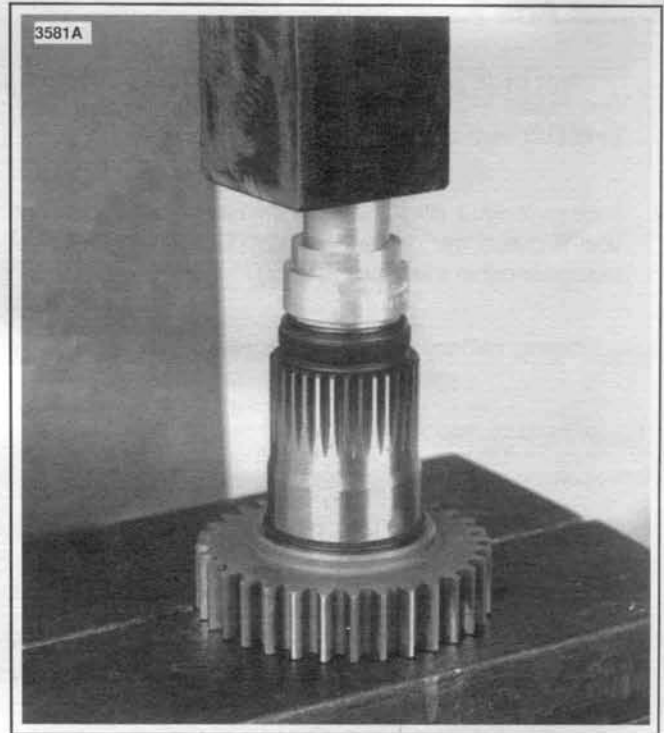
Figure 7-29. Press in Seal
