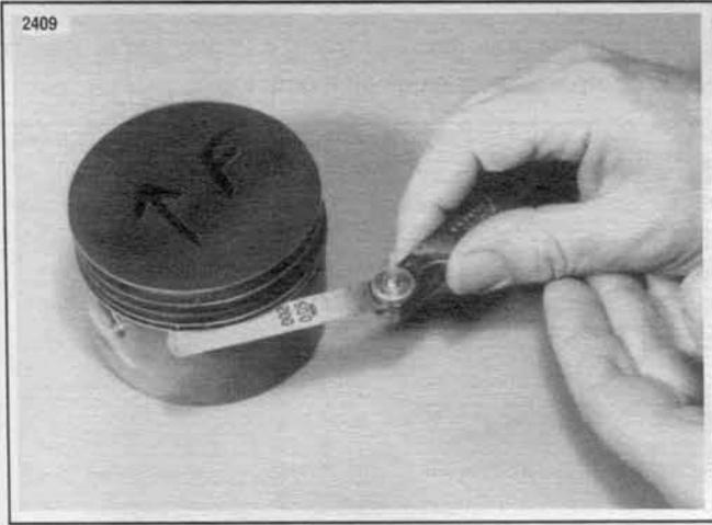
Figure 3-39. Measure Ring Side Clearance
