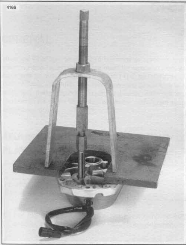
Figure 3-60. Remove Cover Bushing
