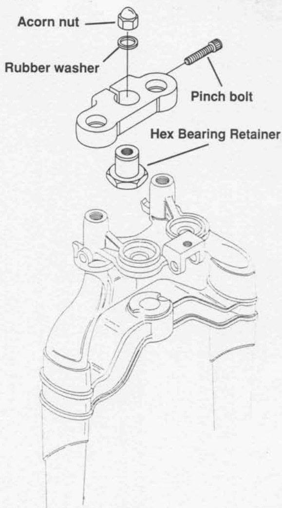
Figure 2-77. Handlebar Risers Assembly
