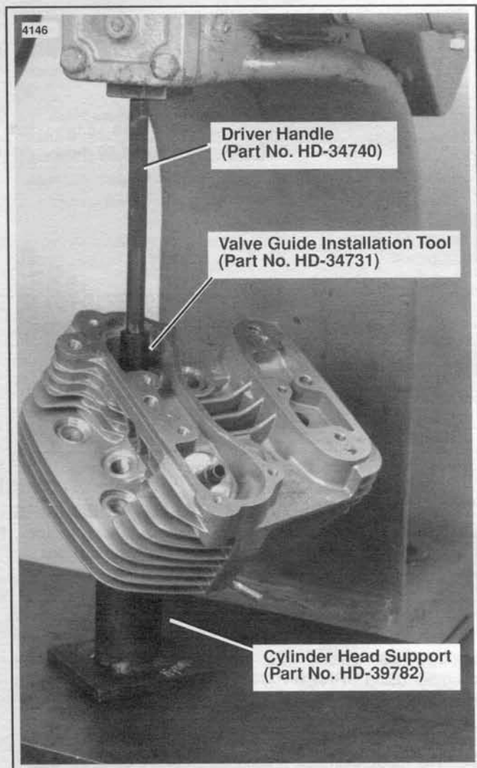
Figure 3-25. Installing Shoulderless Valve Guide
