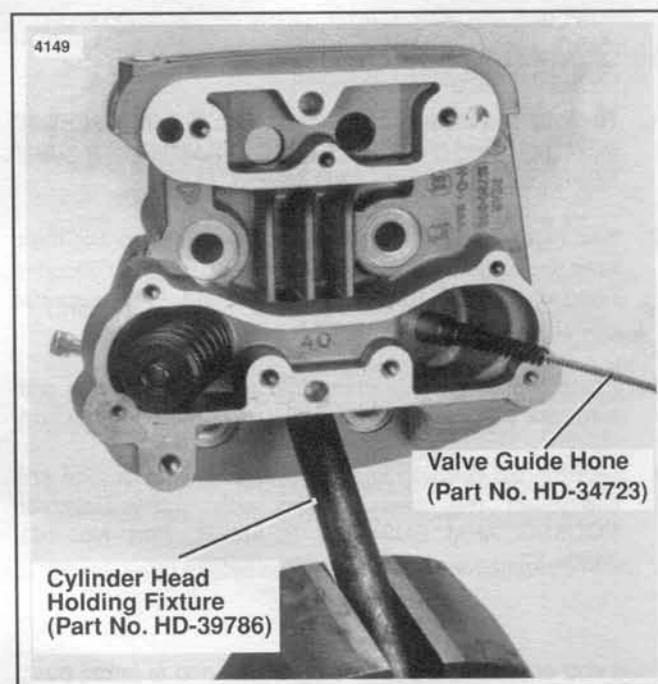
Figure 3-27. Honing Valve Guides
