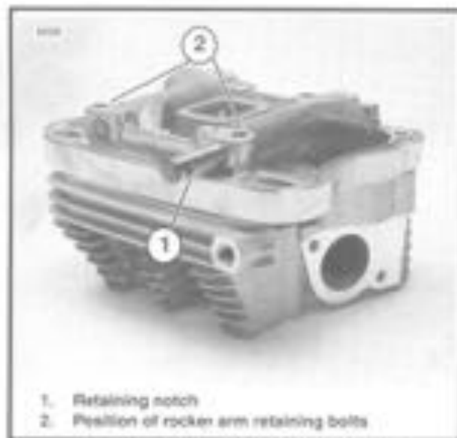
Figure 3-6. Removing Rocker Arm Shafts
