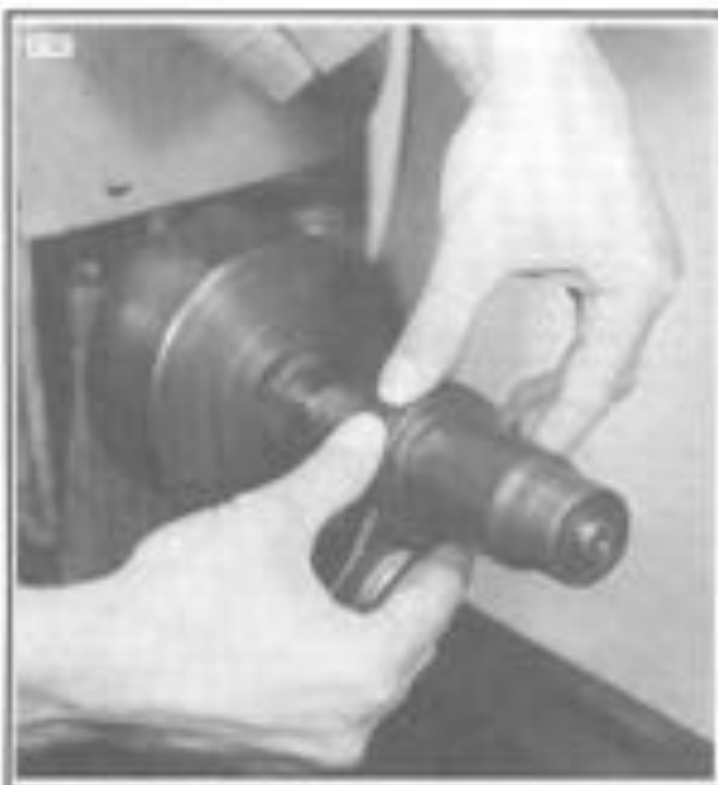
Figure 3-80. Lapping Connecting Rod Races
