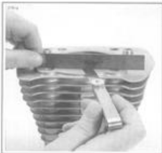
Figure 3-28. Checking Gasket Surfaces
