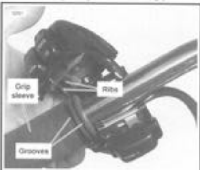
Figure 7-75. Install Left Handlebar Switch Housings
