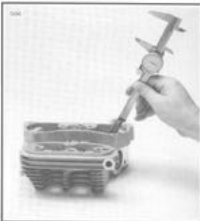
Figure 3-21. Measuring Valve Stem Protrusion
