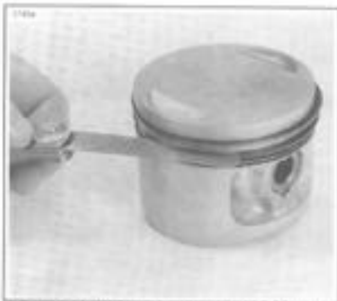
Figure 3-34. Measuring Ring Clearance in Groove
