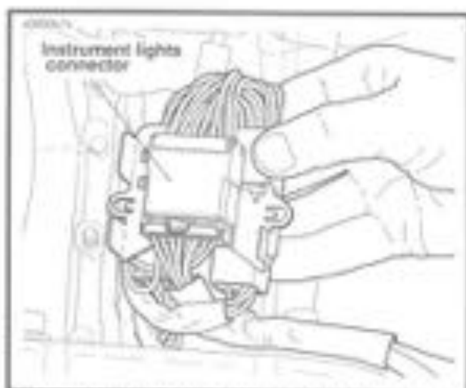
Figure 7-65. XL Custom - Electrical bracket removed
