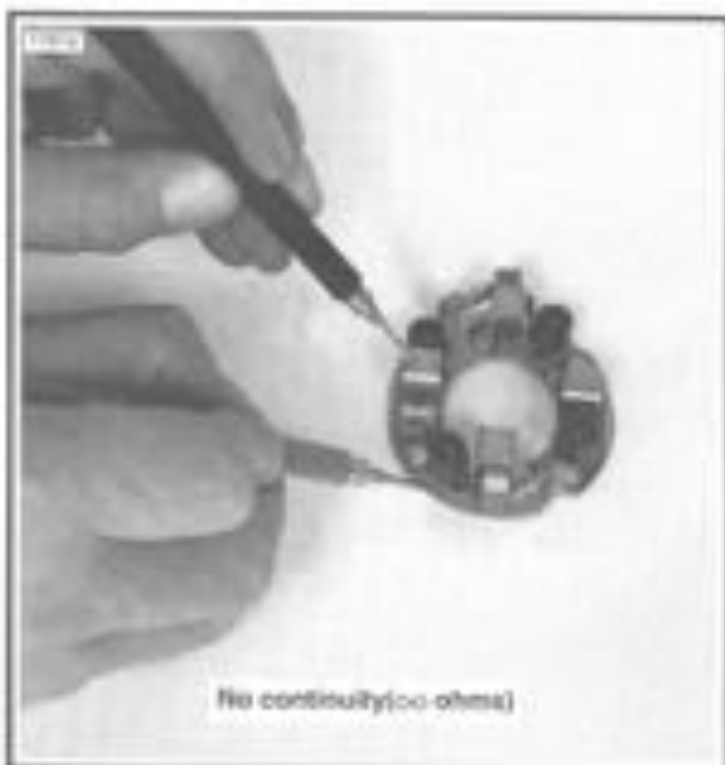
Figure 5-19. Brush Holder Insulation Test
