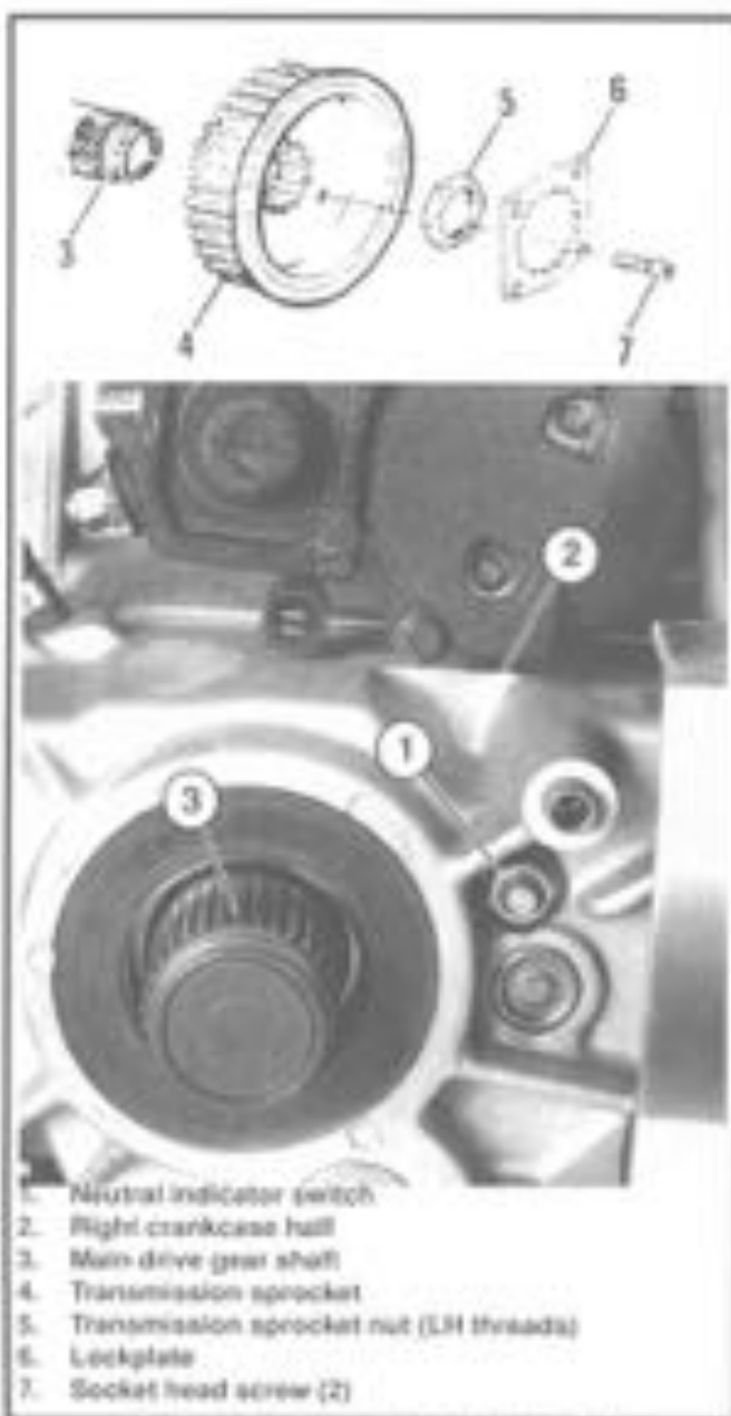
Figure 7-85. Neutral Indicator Switch
