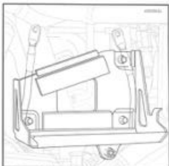
Figure 3-48. Install Battery Tray (Left Side View)
