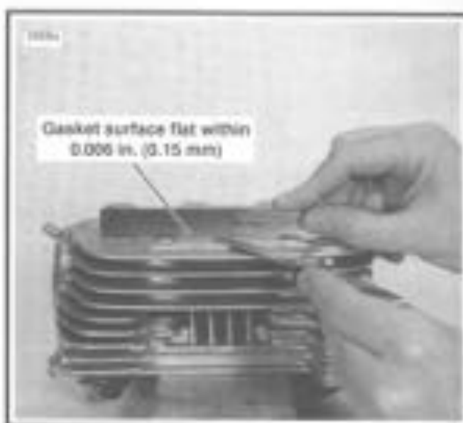
Figure 3-16. Checking Gasket Surface
