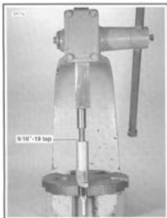
Figure 3-17. Removing Rocker Arm Bushing
