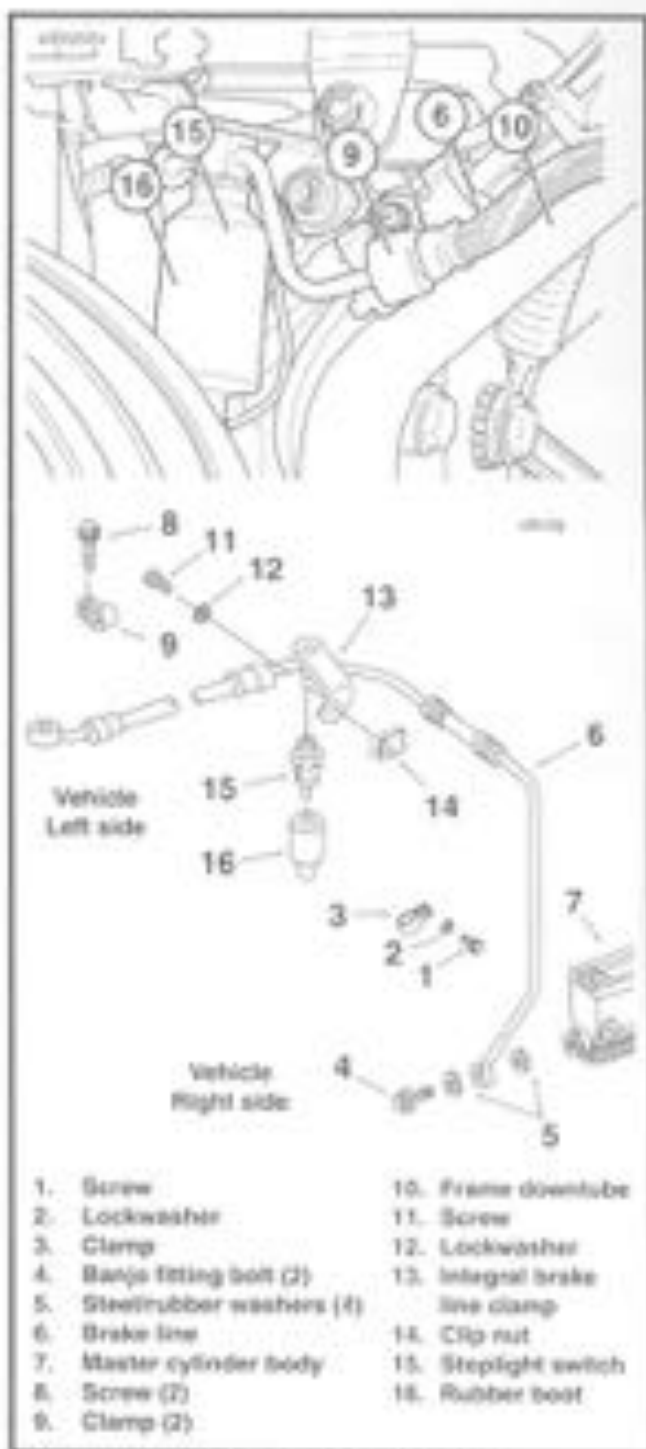
Figure 2-57. Rear Brake Line
