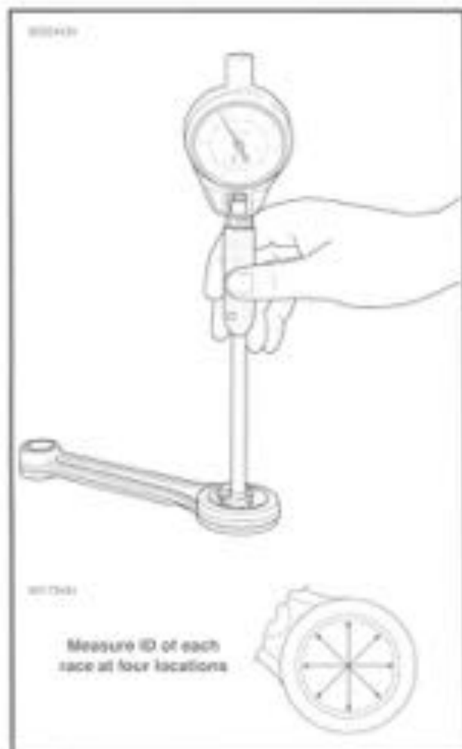
Figure 3-82. Measuring Connecting Rod Race Inside Diameter
