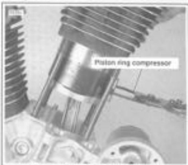
Figure 3-38. Installing Cylinder Over Piston
