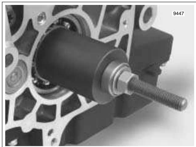
Figure 7-37. Main Drive Gear Installation (Left Side)
