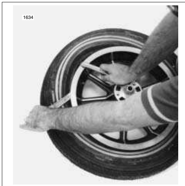
Figure 2-31. Starting Bead Off Rim
