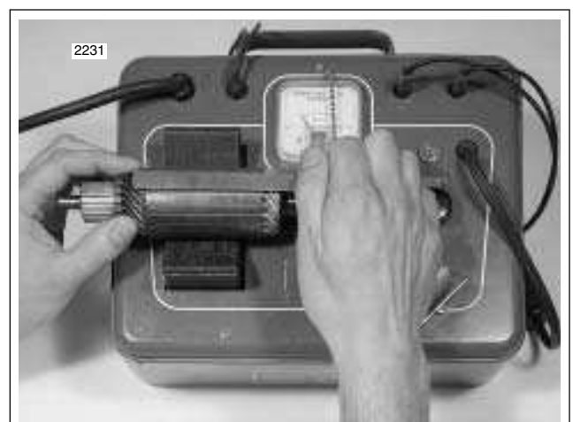
Figure 5-11. Shorted Armature Test Using Growler
