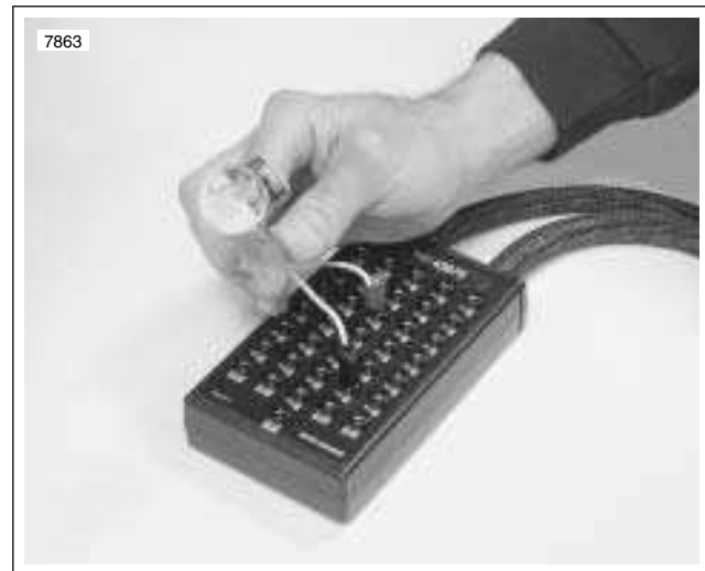
Figure 5-66. Ignition Coil Circuit Test
