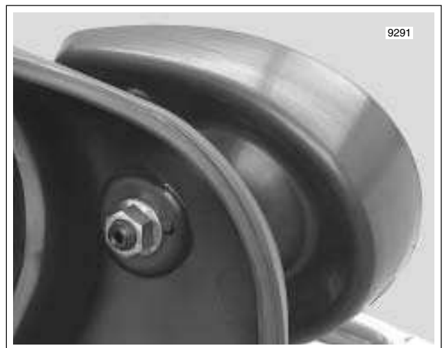
Figure 2-127. Remove Outer Fairing (FLHX)
