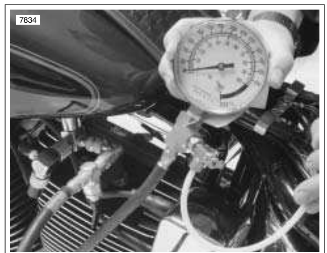
Figure 5-34. Fuel Pressure Gauge Installed (Typical)
