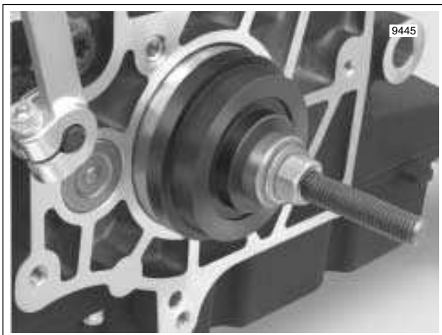
Figure 7-35. Main Drive Gear Bearing Installation (Left Side)
