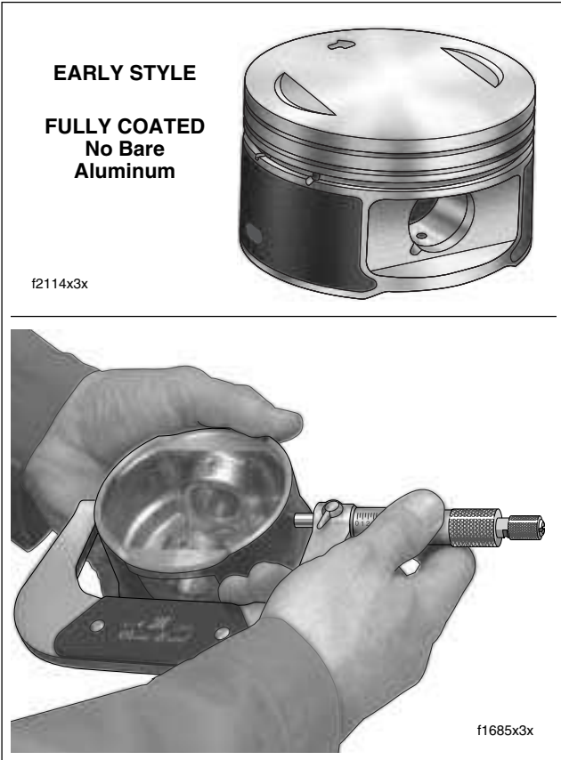
Figure 3-87. Measure Early Style Piston for Running Clearance
