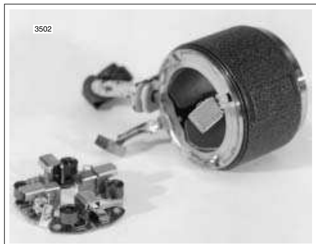
Figure 5-9. Remove Brush Holder
