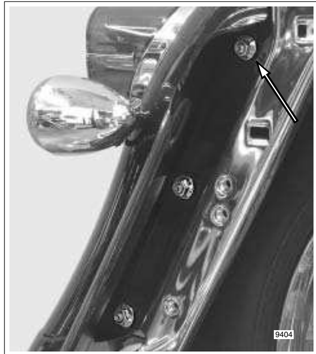
Figure 2-198. Remove Flange Nuts
