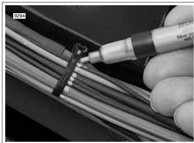
Figure 8-151. Mark Location of Cable Straps
