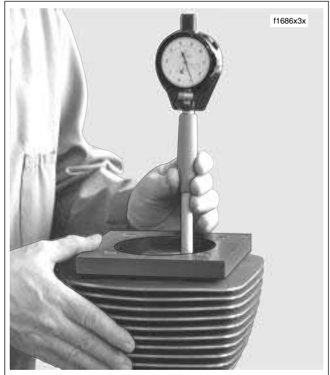
Figure 3-85. Measure for Out-of-Round and Taper
