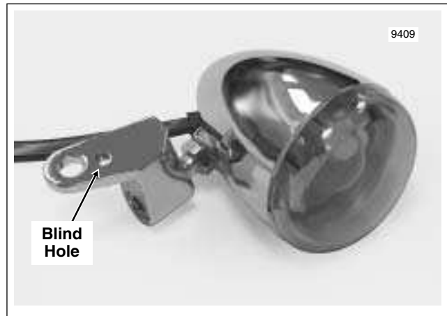
Figure 8-60. Front Left Turn Signal Lamps (FLHRS)
