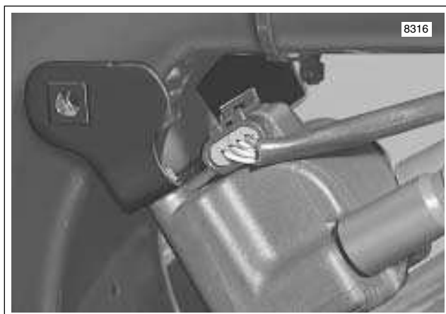
Figure 8-8. Remove Ignition Coil Bracket From Vehicle
