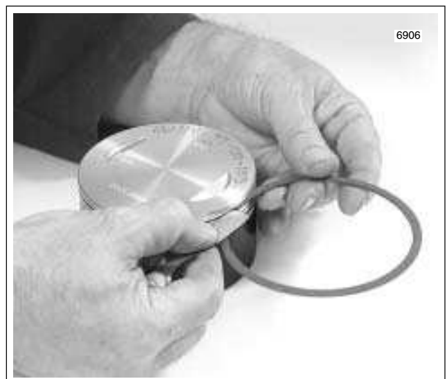
Figure 3-86. Measure Piston Ring Side Clearance
