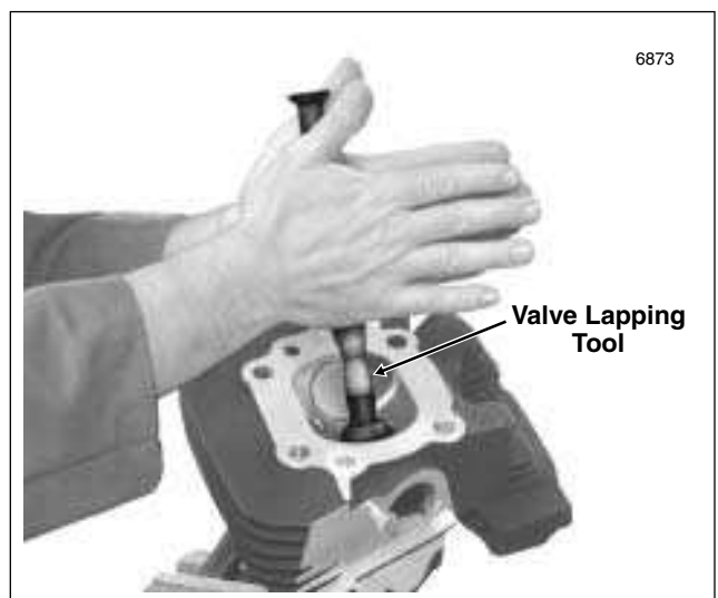
Figure 3-79. Oscillate Tool to Create Contact Area
