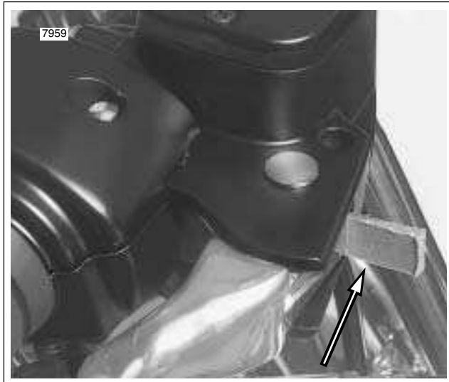
Figure 2-43. Install Cardboard Insert
