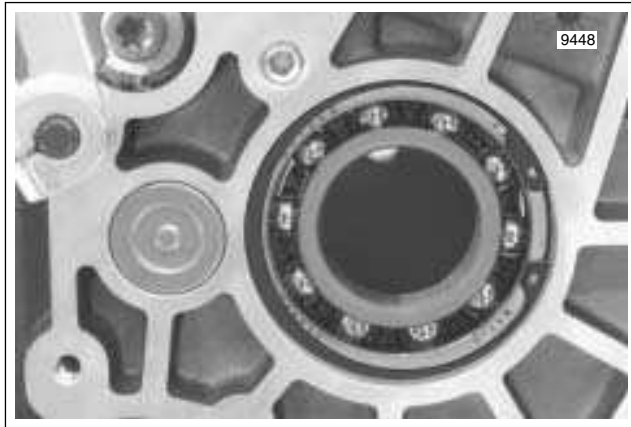
Figure 7-38. Install Retaining Ring With Gap Facing Rear
