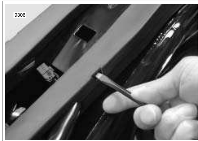
Figure 8-150. Release Catches From Cover
