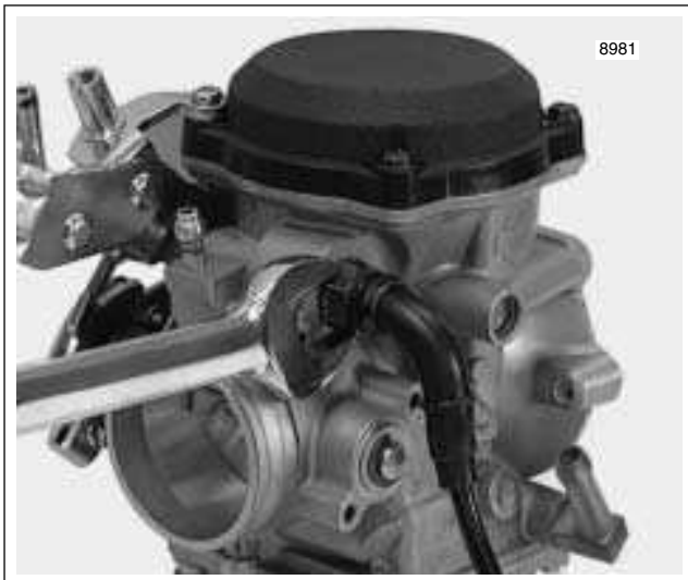
Figure 4-5. Remove Enrichener Cable
