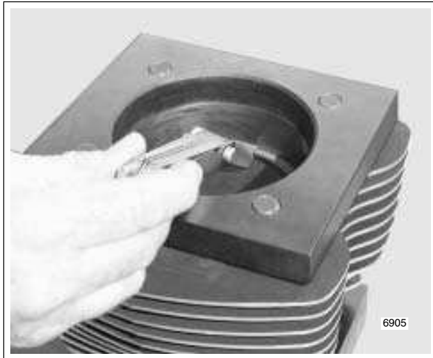
Figure 3-89. Measure Ring End Gap
