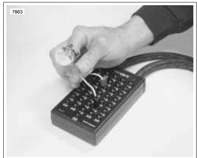
Figure 5-17. Ignition Coil Circuit Test
