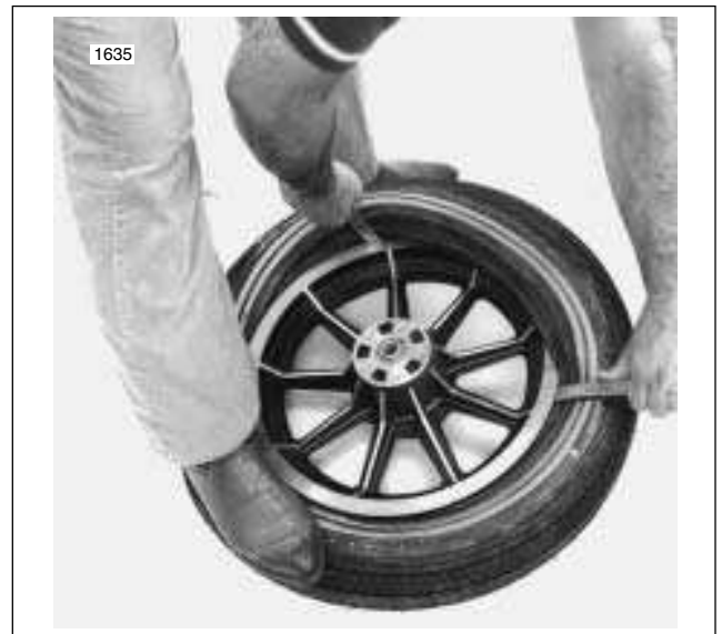
Figure 2-33. Starting Bead on Rim
