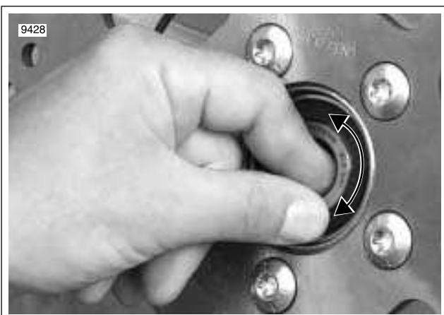
Figure 2-2. Inspect Wheel Bearings
