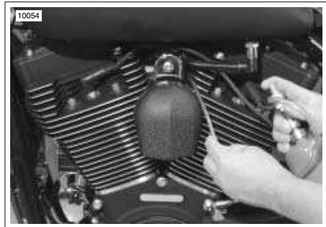
Figure 5-15. Checking for Leaks
