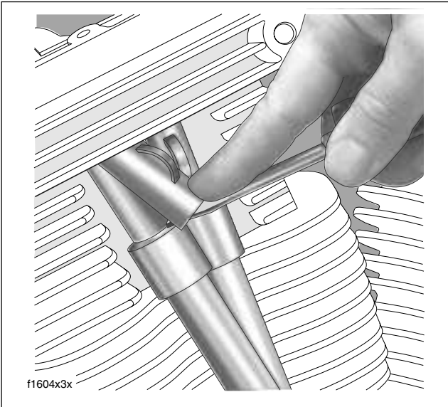
Figure 3-39. Install Spring Cap Retainer
