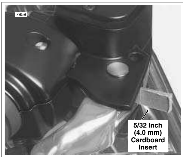
Figure 8-87. Install Cardboard Insert
