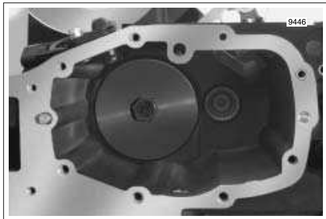
Figure 7-36. Main Drive Gear Installation (Right Side)
