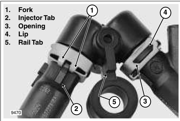
Figure 9-30. Install Spring Clips
