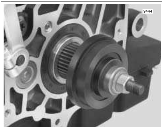
Figure 7-30. Main Drive Gear Removal (Left Side)
