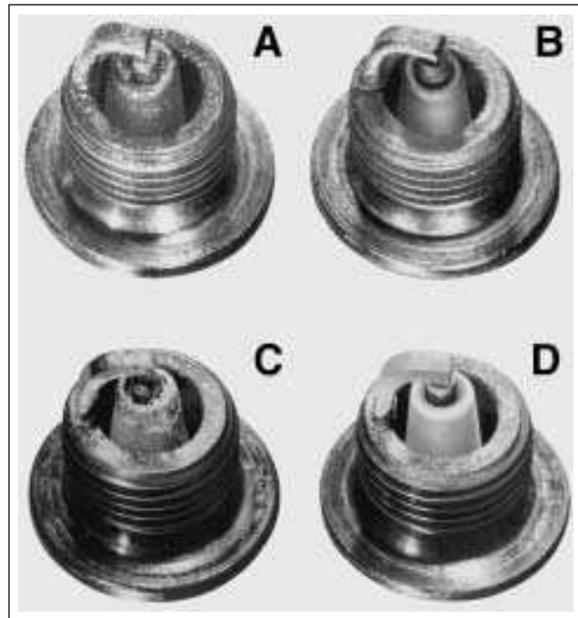
Figure 8-10. Types of Plug Base Deposits
