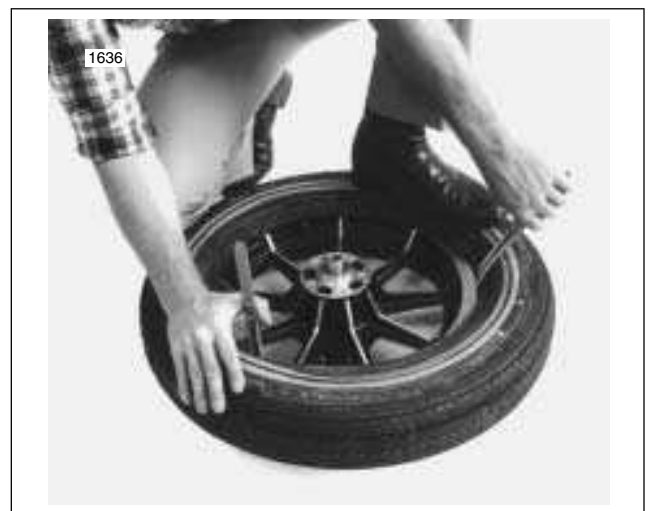
Figure 2-34. Starting Second Bead on Rim
