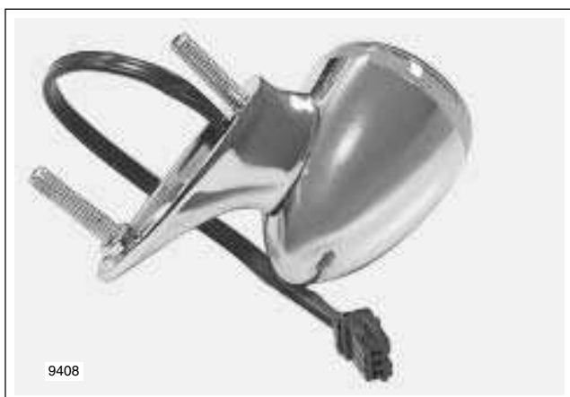
Figure 8-64. Front Turn Signal Lamp (FLTR)
