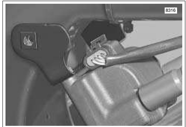
Figure 3-11. Remove Ignition Coil Bracket
