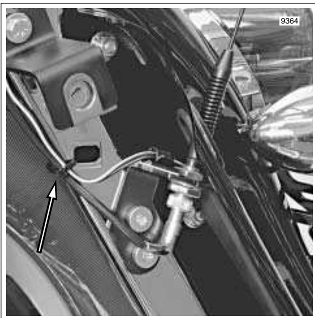
Figure 8-186. Capture Radio Antenna Cable (FLHX)
