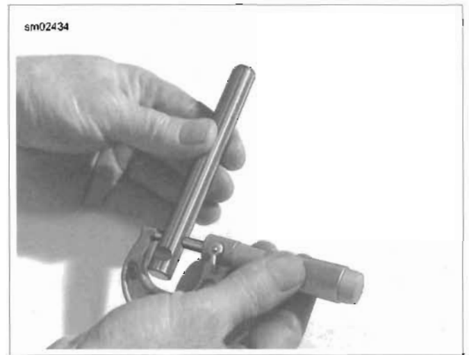
Figure 3-34. Checking Shaft to Bushing Fit
