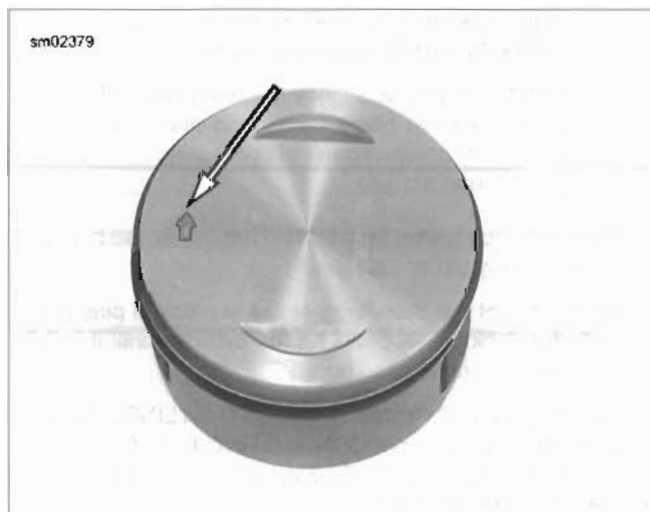
Figure 3-68. Piston Installation Arrow
