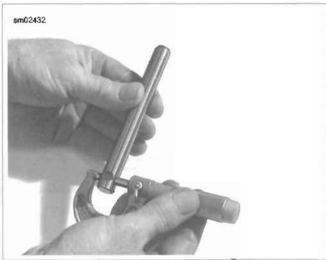
Figure 3-32. Checking Shaft to Support Plate Fit
