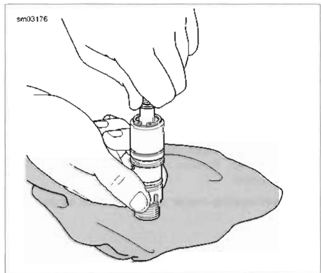
Figure 2-50. Compress Spring and Retaining Ring
