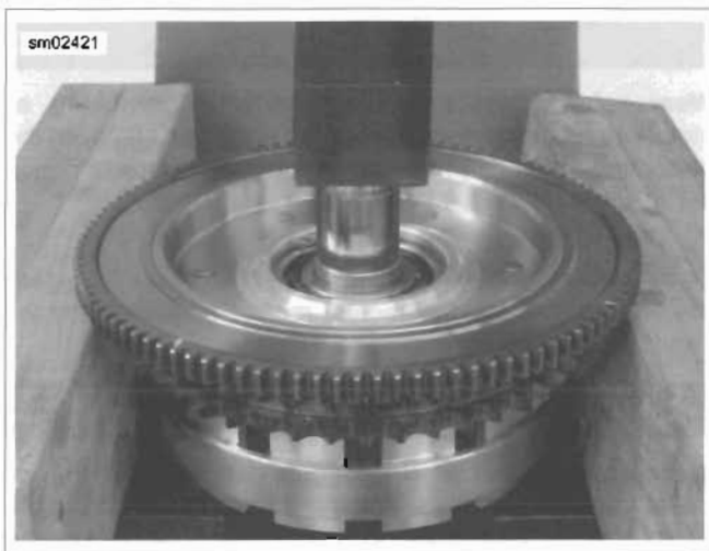
Figure 5-31. Pressing Clutch Hub From Bearing
