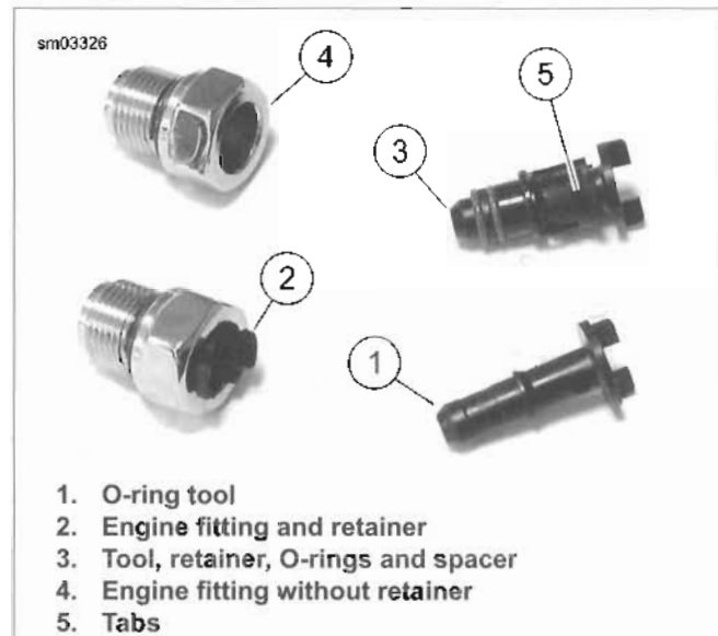
Figure 3-175. Oil Line Retainers (Parts Removed From Engine for Clarity)
