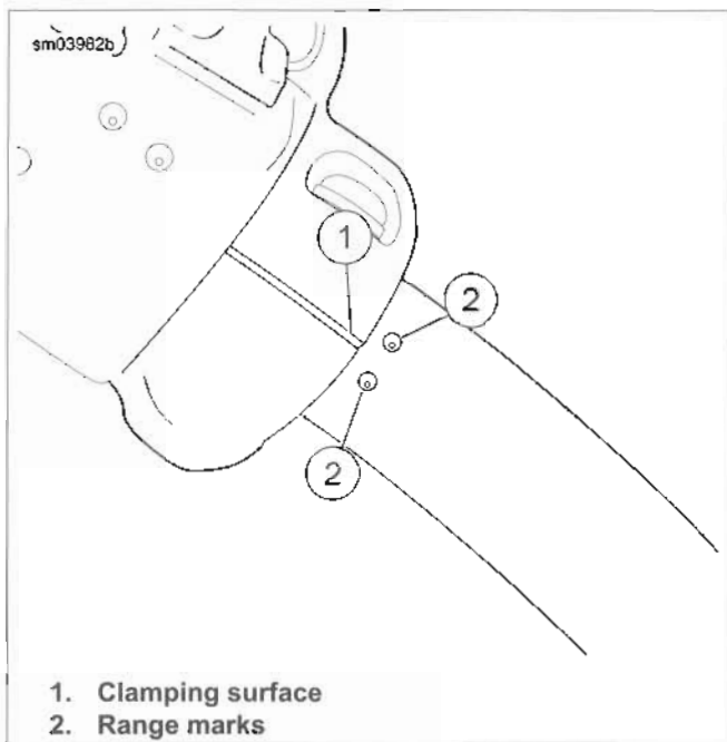
Figure 7-122. Left Hand Control Assembly to Handlebar Alignment
