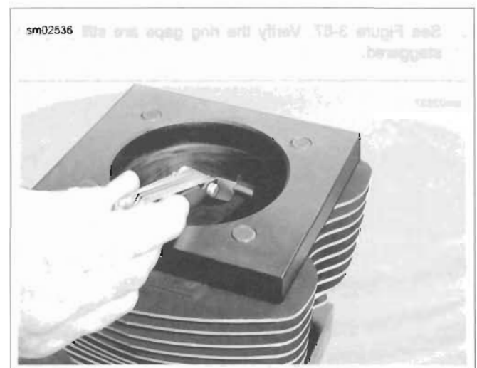
Figure 3-65. Measuring Ring Gap
