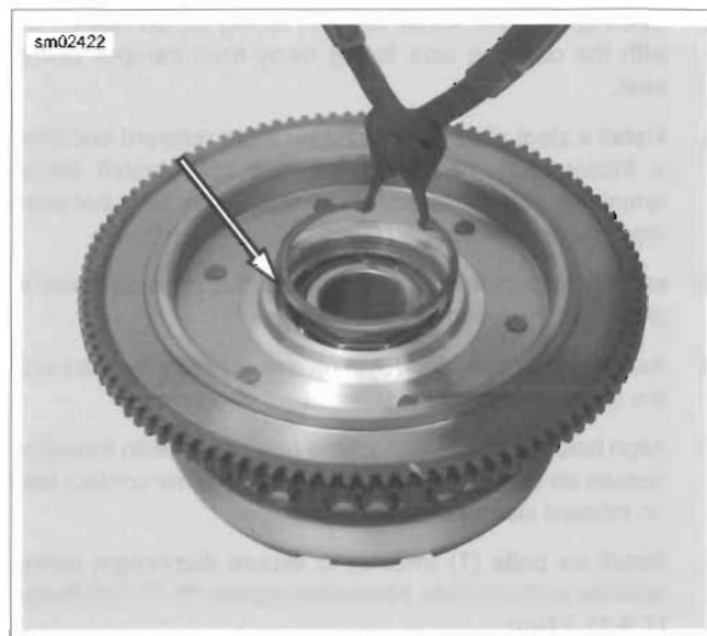
Figure 5-32. Install Clutch Shell Retaining Ring with Flat Side Against Bearing
